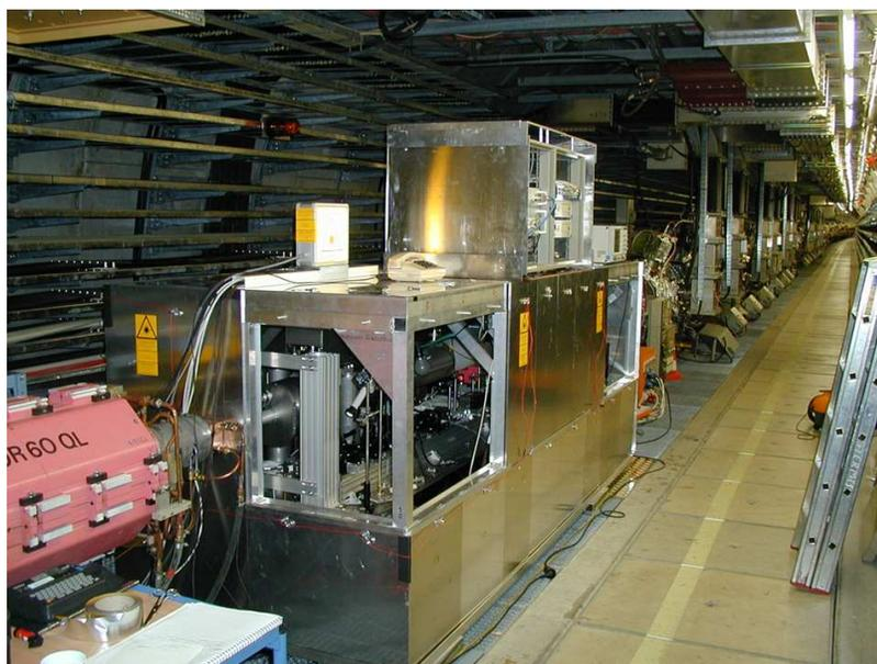
Figure 2.16: Picture of the cavity isotherm and lead shielding house installed in the HERA tunnel in summer 2003.
