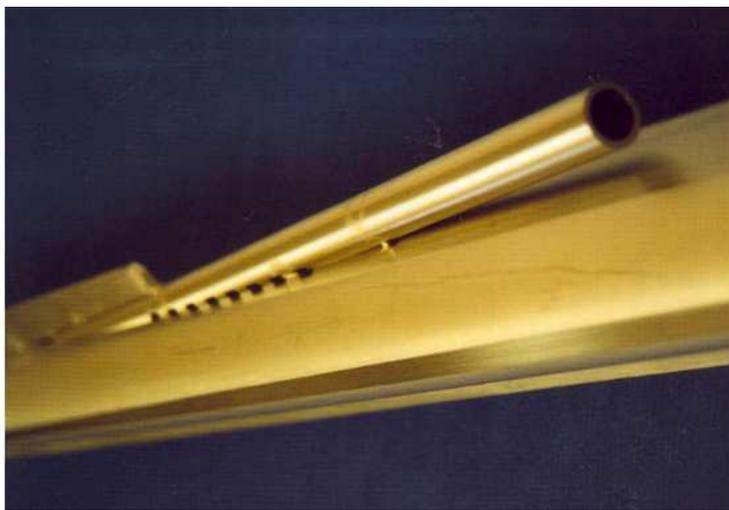
Figure 2.13: Picture of the beam pipe inside the cavity (half is shown). Above the elliptic electron beam pipe, a circular tube is soldered to reduce wake-field excitations. The small holes visible on the picture have been implemented for vacuum conductance purposes between the cavity and the beam pipe.
