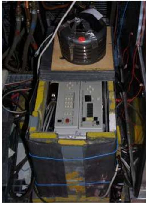
Figure 2.19: Picture of the shielding of the laser controller (top picture), of the controller of the entrance quarter wave plate rotating mount (bottom left picture), and of the controllers of the motorised cavity alignment mirrors (bottom right picture).
