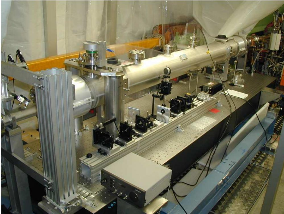
Figure 2.12: Picture of the cavity taken during the installation in the tunnel. The laser and the optical components before the cavity entrance are located on a rail parallel to the cavity vessel.
