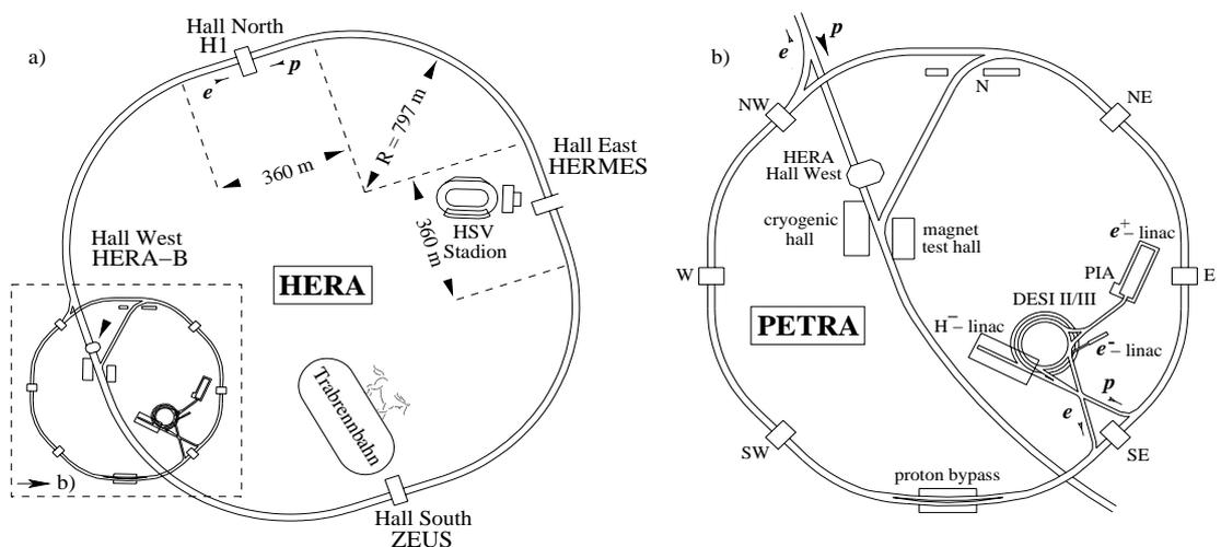
Figure 2.1: The geometry of the HERA collider a) and its pre-accelerators b).
