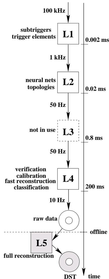
Figure 2.6: The H1 Trigger System.
