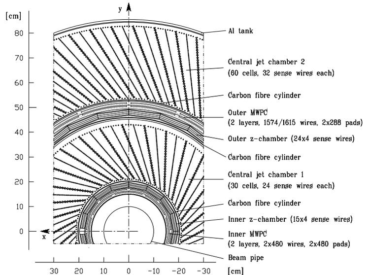
Figure 2.3: The  $(x, y)$  plane wire structure of the CJC .
