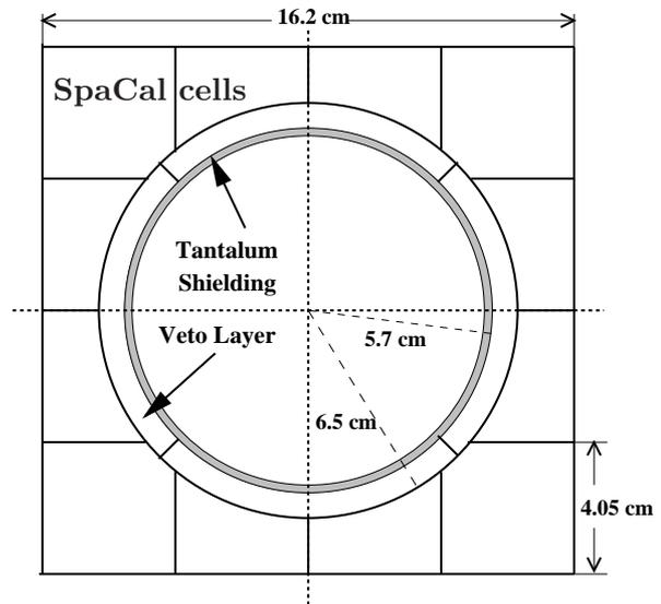
Figure 3.14: The  $(x, y)$  view of the SpaCal inner cells and the VETO layer.
