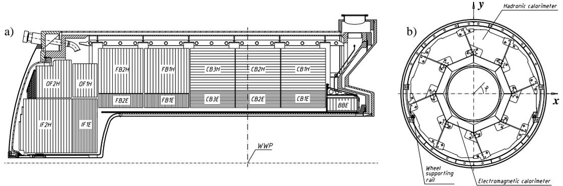
Figure 2.4: The Liquid Argon calorimeter; a) longitudinal and b) transversal section in the central region.
