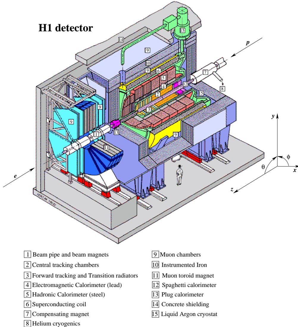
Figure 2.2: The H1 detector architecture.
