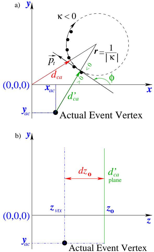
Figure C.1: Definition of track parameters in the  $(x, y)$  plane and of  $d'_{ca}$ .
