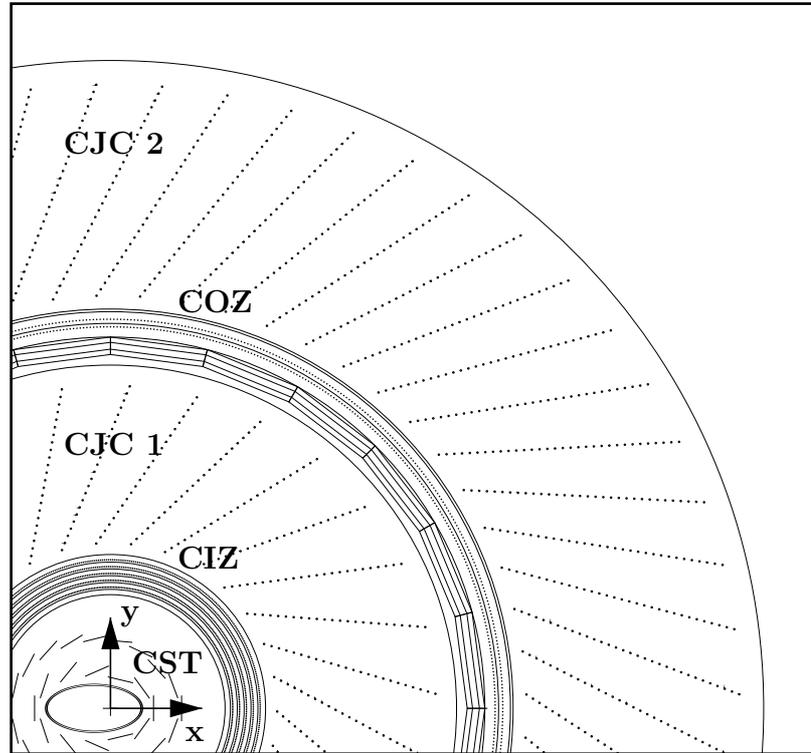
**Figure 1.3:** *Cross section of the tracking system in the  $x$ - $y$  plane. The axes originate from the interaction point. The central jet chamber CJC 1 and 2 are indicated as well as the central inner (CIZ) and outer (COZ)  $z$ -chambers and the central silicon tracker (CST).*
