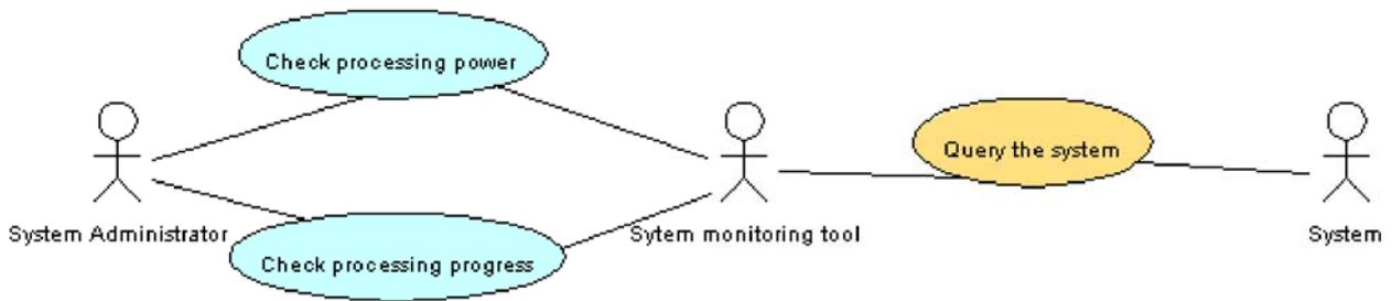
Fig. 11 . System monitoring use case diagram
