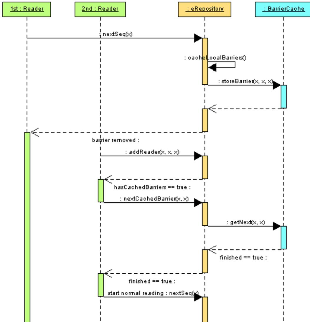
Fig. 23 . Reading cached barrier sequence diagram
