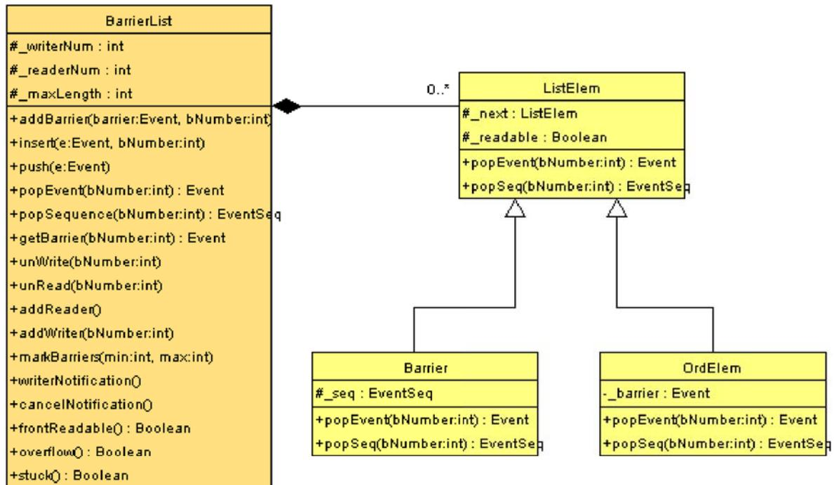
Fig. 17. Barrier list class diagram.
