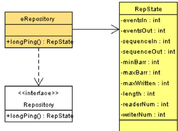
Fig. 18 . Repository state class diagram.
