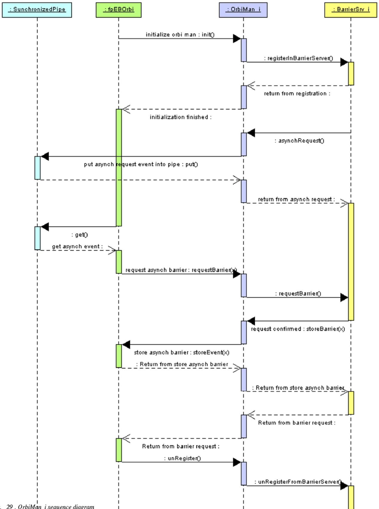
Fig. 29 . OrbiMan\_i sequence diagram
