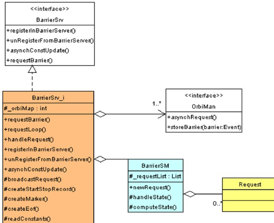
Fig. 30 . Barrier server class diagram
