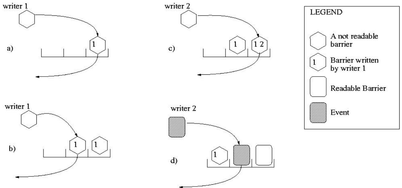
Fig. 21. Barrier list with two writers.
