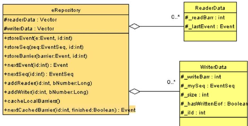
Fig. 16 . Repository class diagram with client data classes
