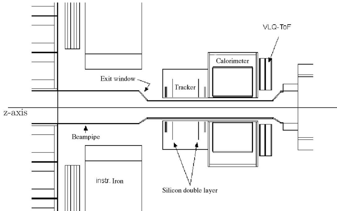
**Figure 3.2:** Side view of the VLQ spectrometer and the modified beampipe implemented in the simulation of the H1 experiment.
