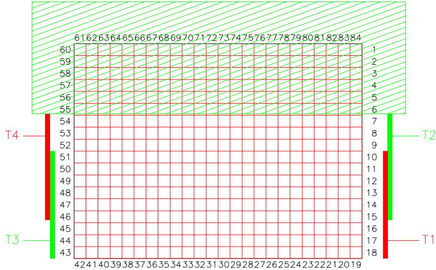
**Figure 5.1:** Schematic view of the sliding window scheme of the VLQ trigger for the upper module. The trigger segments T1 and T2 (T3 and T4) on the right (left) of the calorimeter each combine 9 readout channels with an overlapping region of 6 channels. The shaded area shows the region which is not included in the trigger.
