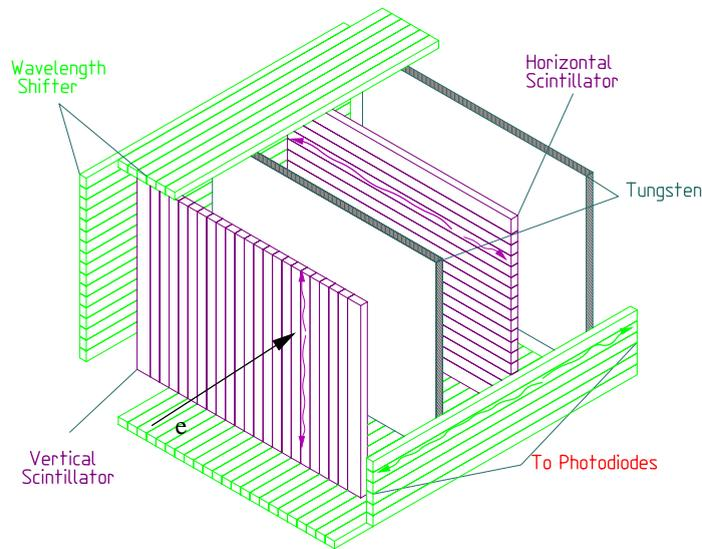
**Figure 2.8:** Schematic layout of a VLQ calorimeter.
