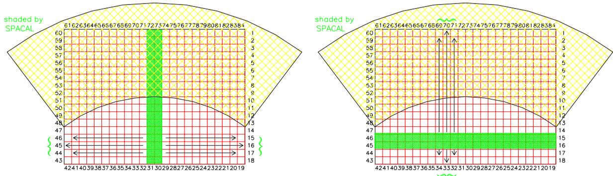
**Figure 4.11:** Channel-to-channel calibration procedure for the vertical (left) and for the horizontal scintillator array (right). The channels are numbered [1:84]. For the calibration procedure, events inside the gray bands are selected.
