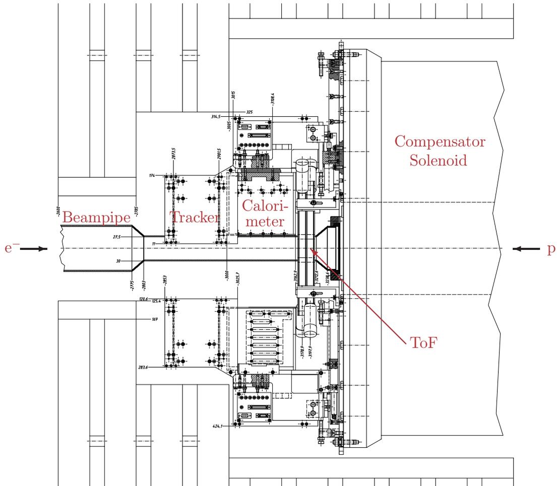
**Figure 2.7:** Schematic layout of the VLQ spectrometer. The upper module is shown in the data taking position and the lower module in the parking position.
