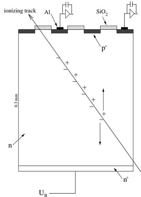
**Figure 2.9:** Principle of a silicon microstrip detector.
