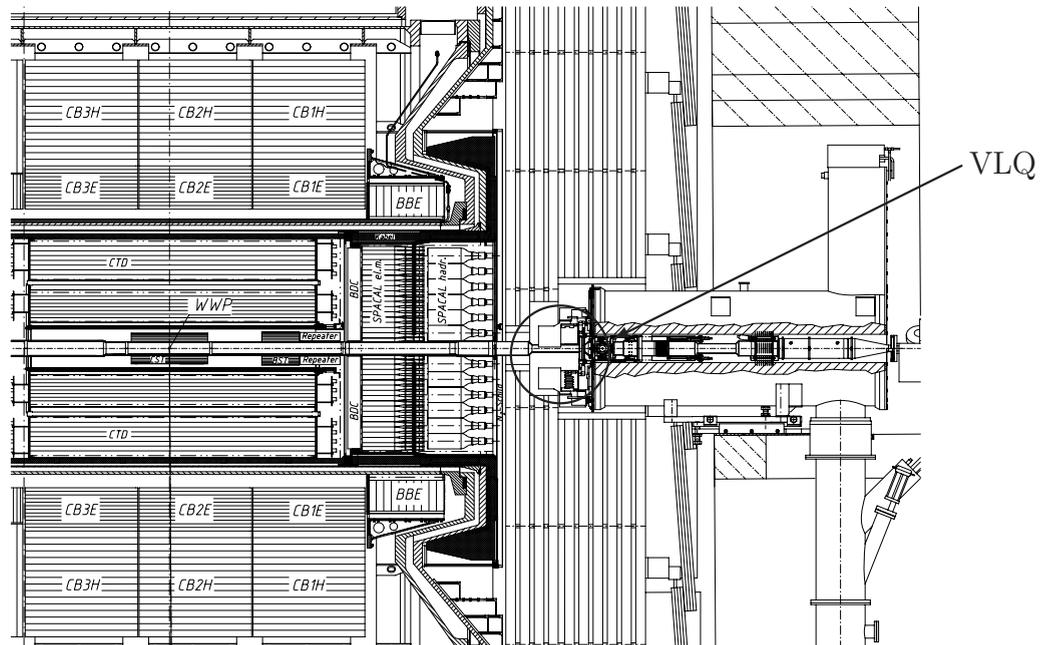
**Figure 2.6:** Longitudinal cut of the backward region of the H1 detector including the VLQ spectrometer. The upper module is shown in data taking position close to the beampipe, whereas the lower module is in the parking position behind the instrumented iron. WWP denotes the nominal interaction point.
