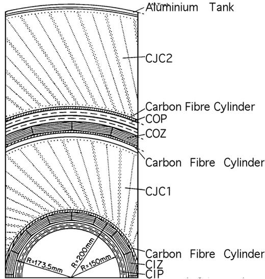
Figure 2.4: A section through the  $r - \phi$  plane of the central tracking detector.
