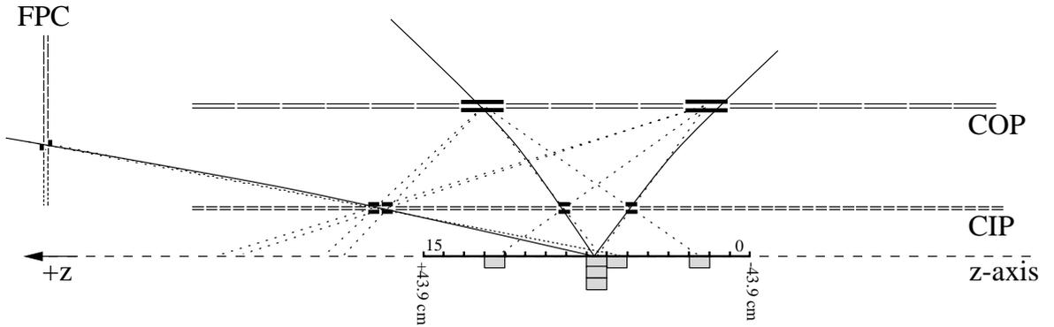
Figure 2.6: A schematic representation of the filling of the  $z$ -vertex histogram. All possible rays for the hit pattern are shown. The true rays are shown in bold and are linked to the significant  $z$ -vertex histogram peak.
