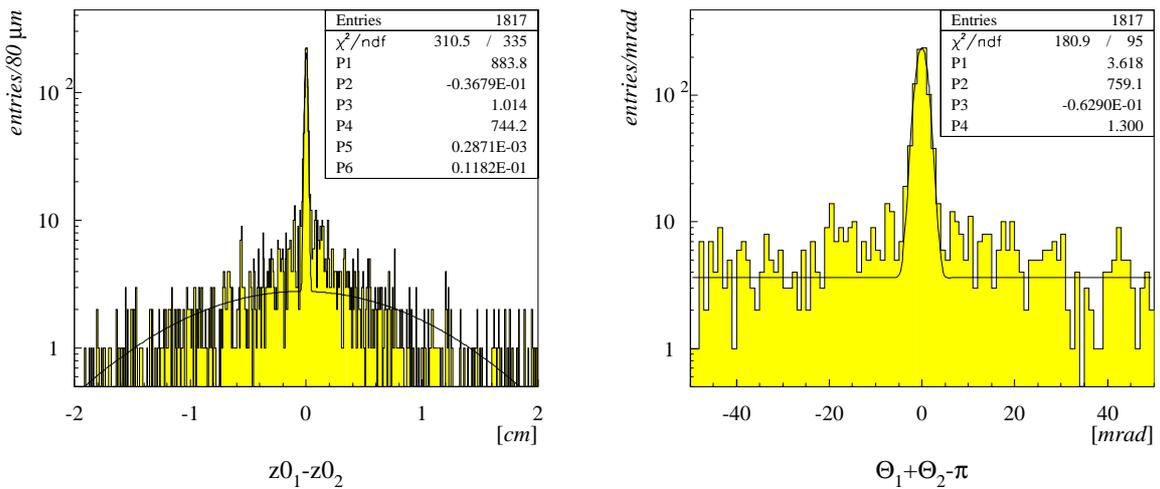
Figure 4.20: Cosmic track parameters measured by the CST in  $R$ - $z$ . Two normalized Gaussians (P1-P3 and P4-P6) have been fitted to the  $z_0$ -distribution (left) and a Gaussian (P2-P4) plus a constant term (P1) to the  $\Theta$ -distribution (right).
