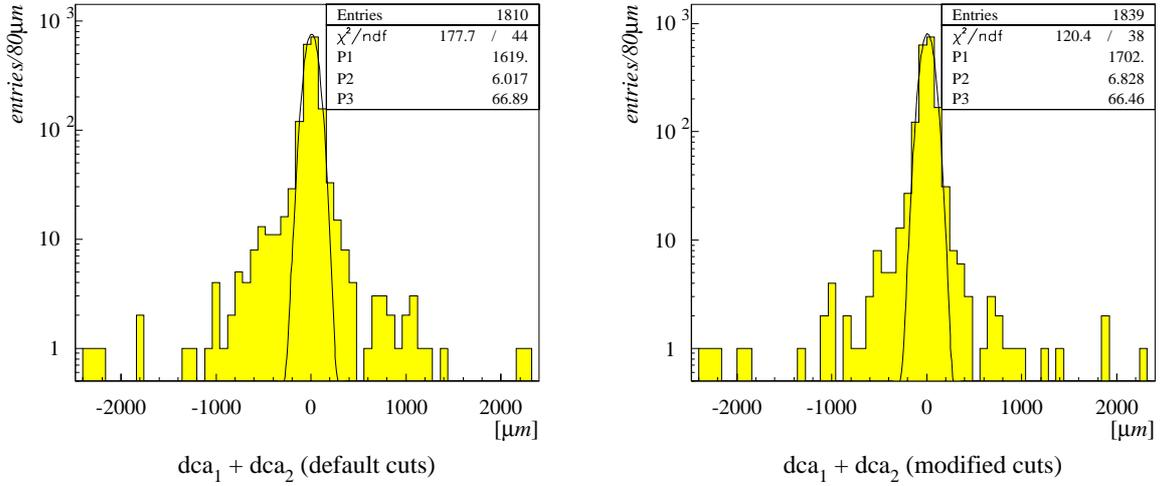
Figure 4.16: Improvement of the  $p$ -side link-efficiency by raising the cluster significance cut. The histograms (log scale) show the  $dca$ -sum distributions of the CST fitted tracks with the default cuts for the linking (left) and with the modified cut values (right) with normalized Gaussians fitted to them.
