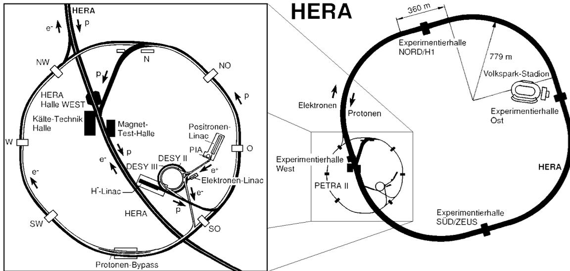
Figure 2.1: The electron-proton collider HERA. The zoomed view on the left displays the injectors and pre-accelerators while the storage ring itself with the four experiment areas is shown on the right. The H1 experiment is situated in the north section of the ring.
