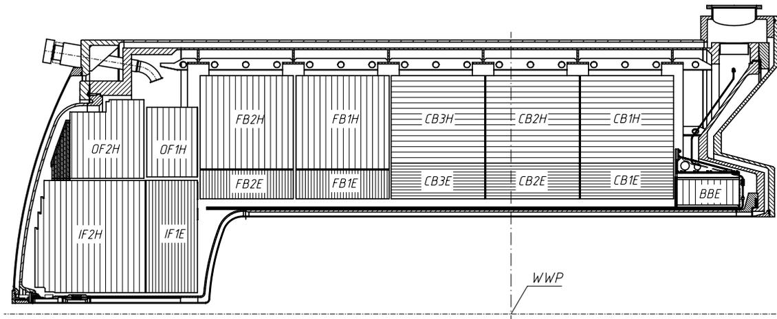
Figure 2.4: Side view of the liquid argon calorimeter showing a cross-section of the eight wheels (left to right). The protons enter from the right, WWP denotes the nominal interaction point.
