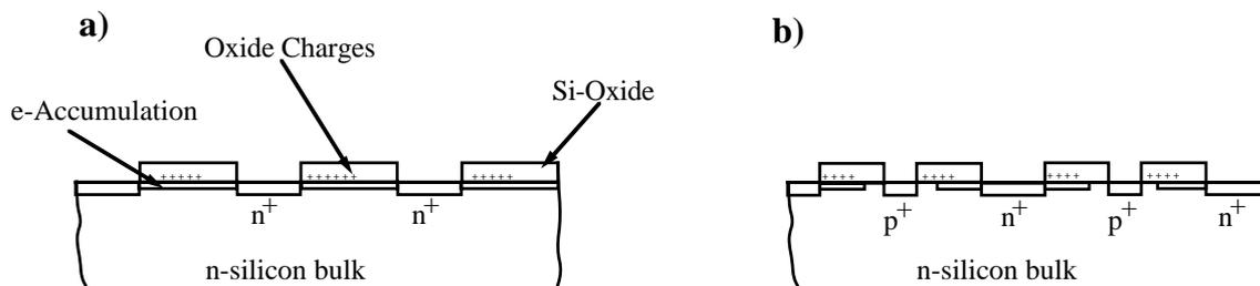
Figure 2.10: *The use of p-blocking implants for isolating n-side strips (from [32]):*
