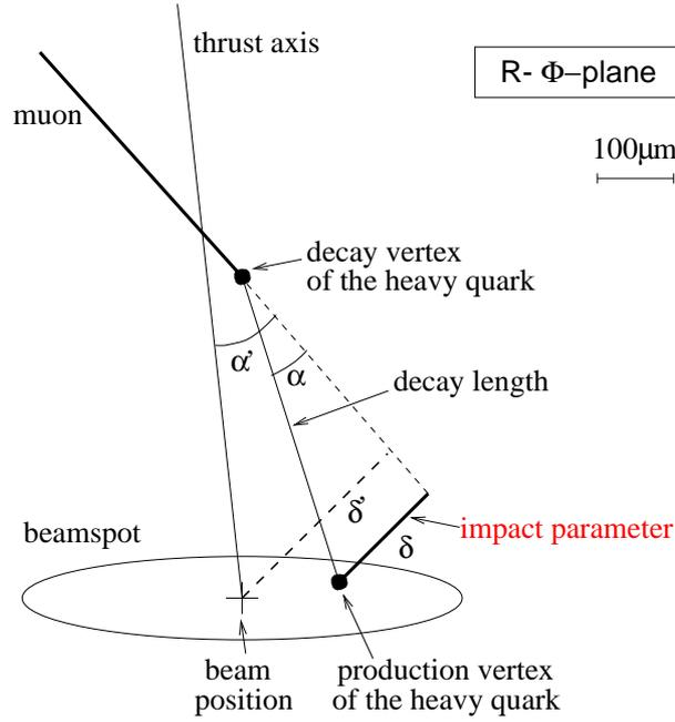
Figure 5.8: *Impact parameter method.* The heavy meson is produced at the primary vertex within the beamspot. It decays semi-leptonically into a muon with angle  $\alpha$  and impact parameter  $\delta$ . In the measurement, the flight direction of the heavy meson is approximated by the thrust axis, and the primary vertex by the nominal beam position resulting in the quantities  $\alpha'$  and  $\delta'$ <sup>1</sup>.
