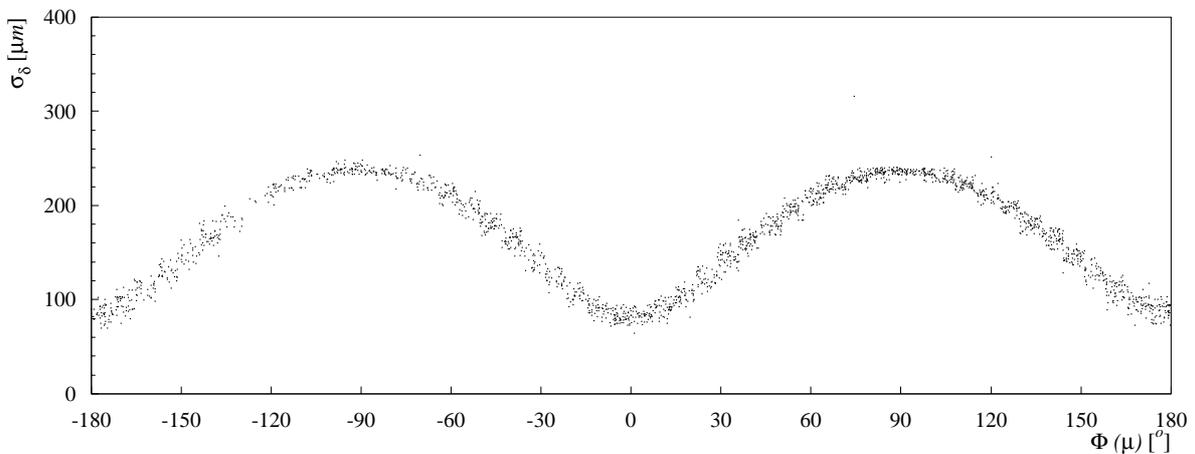
Figure 5.12: *Error on the impact parameter vs.  $\Phi$ . The dependence on the dimensions of the beamspot is clearly visible: the error is largest for  $\Phi = \pm 90^\circ$  where the beamspot size in  $x$ -direction of  $\sigma_x \approx 180 \mu\text{m}$  is relevant. The error is determined for selected muon tracks (s. next section) by means of error propagation for  $dca'$  (Eq. (5.8))*
