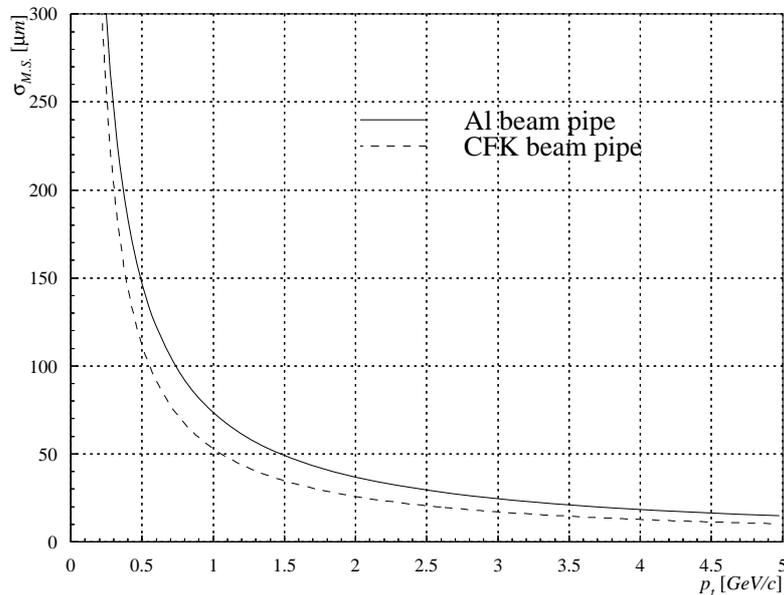
Figure 2.12: *Vertex resolution as function of transverse momentum. Only the contribution from multiple scattering in the beam pipe is plotted.*
