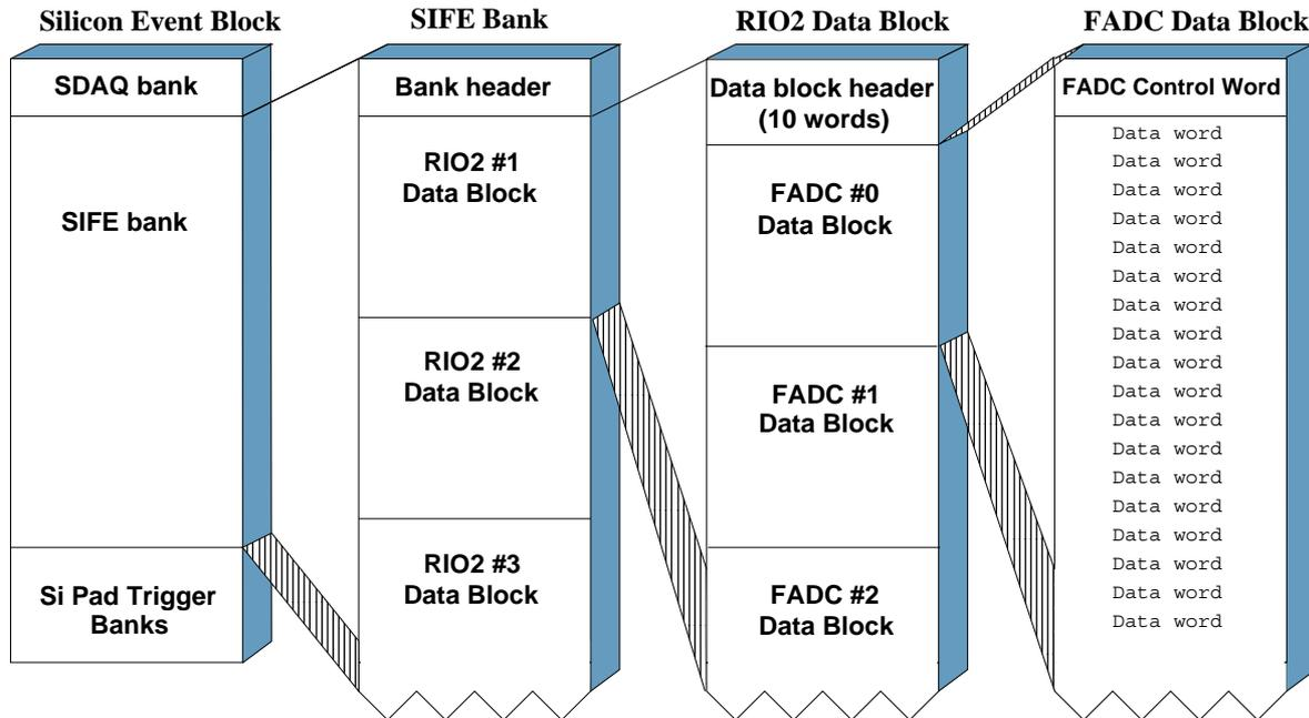
Figure 3.4: Structure of a Silicon event data block
