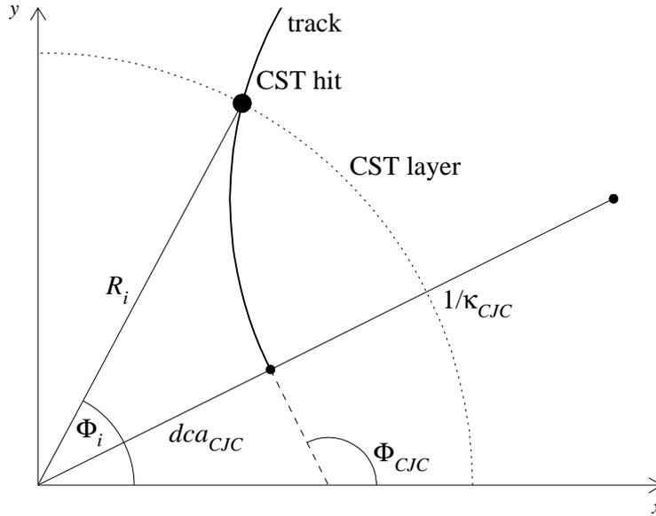
Figure 4.9: *Track and spacepoint parameters in the  $R$ - $\Phi$ -plane (=  $x$ - $y$ -plane). A track parameterized by the variables  $\kappa_{CJC}$ ,  $\Phi_{CJC}$ , and  $dca_{CJC}$  crosses a CST layer (indicated by the dotted line) where the measured hit has the coordinates  $R_i$  and  $\Phi_i$ .*
