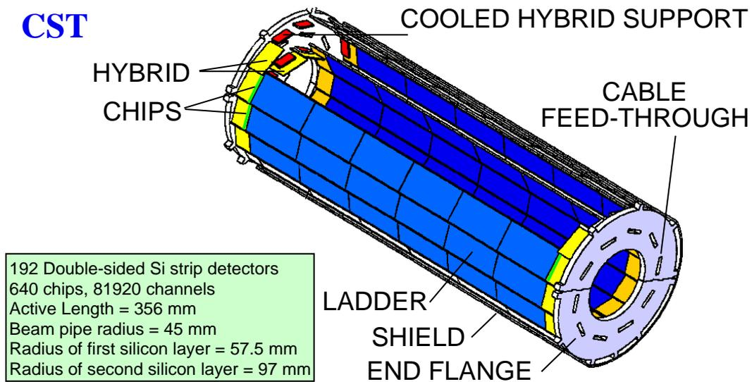
Figure 2.8: *The microvertex detector CST*
