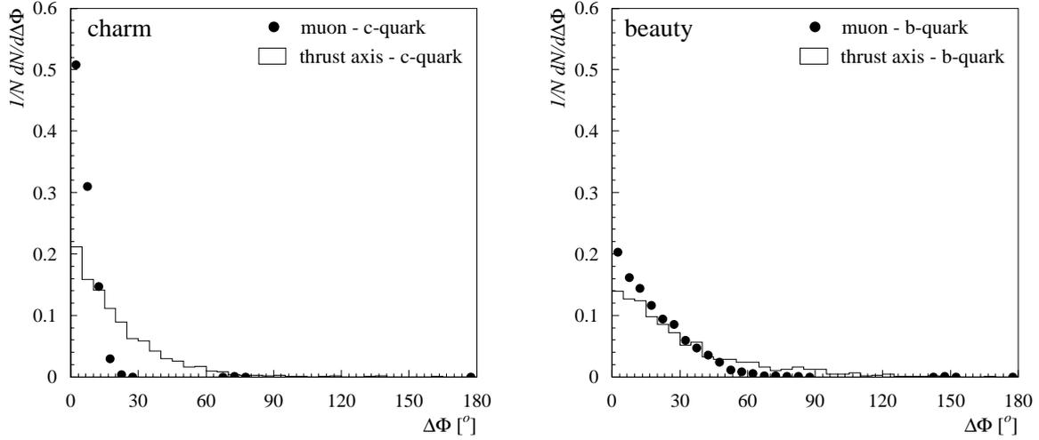
Figure 5.10: Opening angle (in the  $R$ - $\Phi$ -plane) between generated heavy quark direction and reconstructed muon (dots) and reconstructed thrust axis (histograms) for  $c\bar{c}$ - (left) and  $b\bar{b}$ -events (right).
