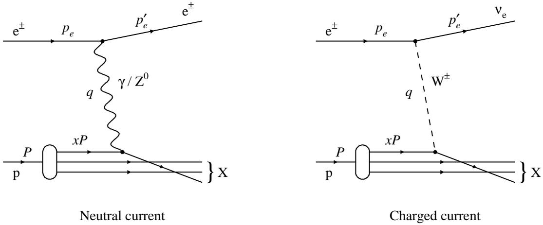
Figure 1.1: Feynman graphs for neutral-current and charged-current electron-proton scattering
