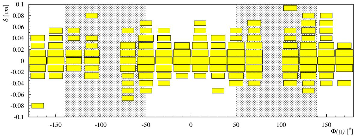
Figure 5.20: Correlation of  $\delta$  and  $\Phi(\mu)$ . The shaded regions indicate the  $\Phi$ -range where the error on  $\delta$  is large due to the larger beam spot extension in  $x$ -direction. The “holes” at  $\Phi = \pm 90^\circ$  are due to the cut of  $\sigma_\delta < 230\mu\text{m}$ , cf. Chap. 5.3.2.
