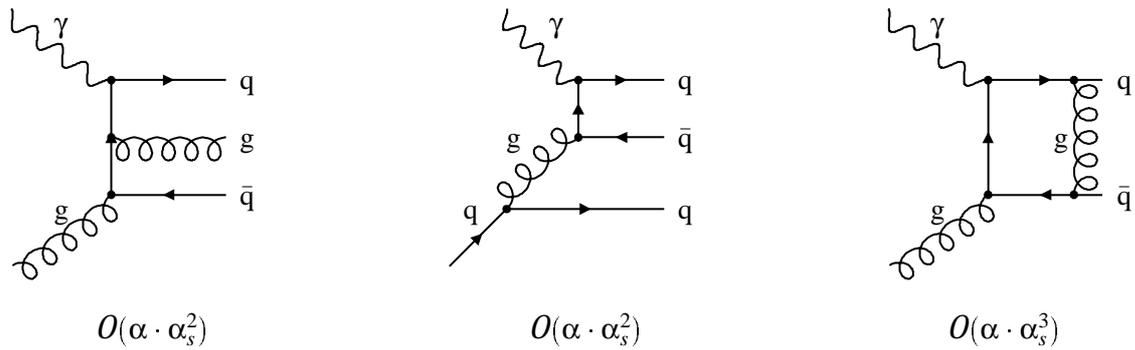
Figure 1.4: Higher order processes of heavy quark photoproduction (direct component)
