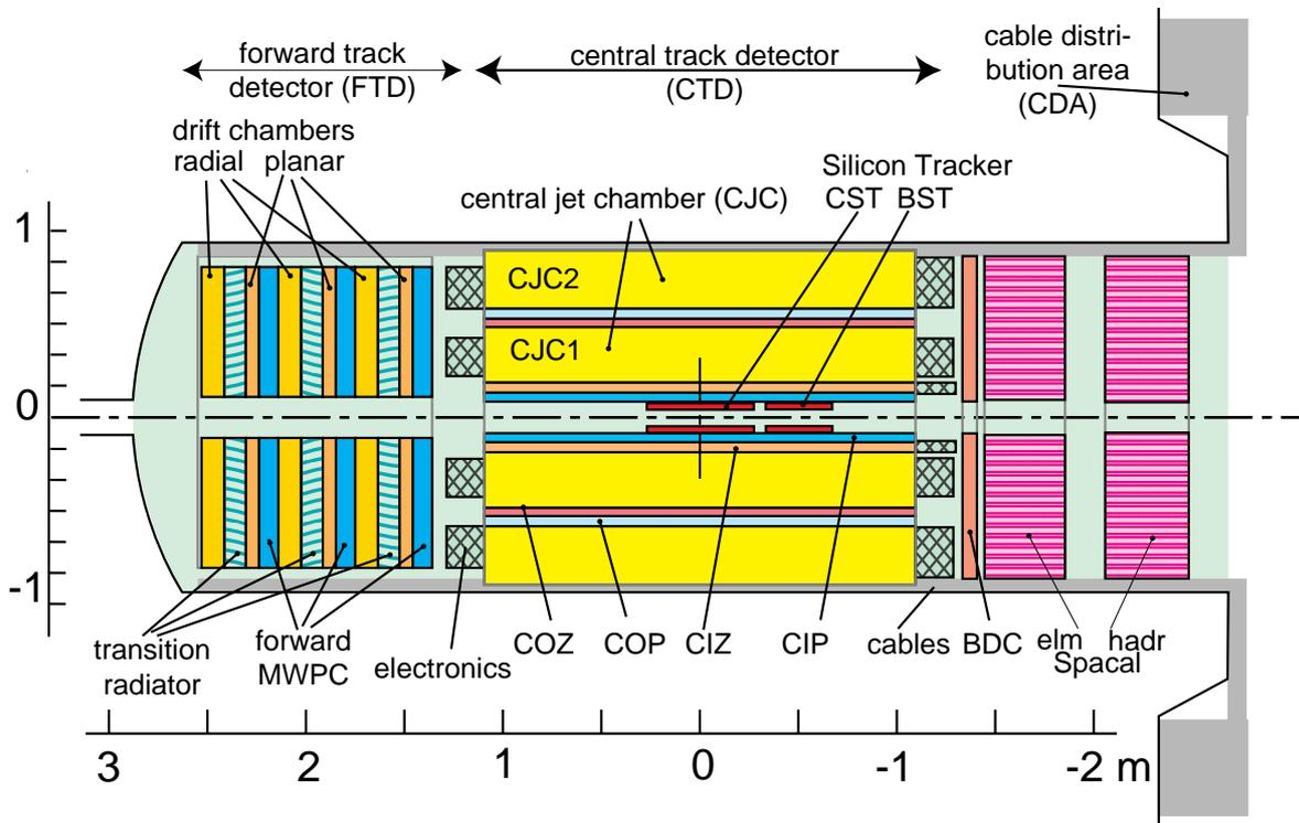
Figure 2.3: Side-view of the tracking detectors
