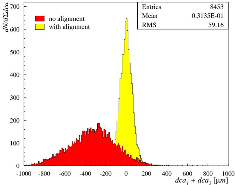
Figure 4.3: *Effect of applying alignment corrections to CST measurements. Dark histogram:  $dca_1 + dca_2$ -distribution for CST tracks without alignment corrections, light histogram: same tracks calculated with corrected coordinates for the CST measurements.*
