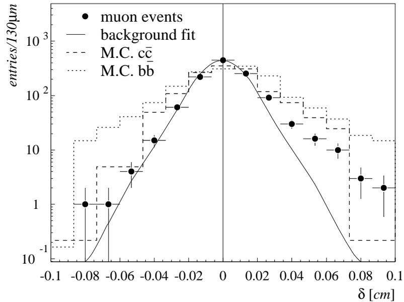
Figure 5.17: Impact parameter distributions for muon data and the  $c\bar{c}$ - and  $b\bar{b}$ -Monte Carlo samples. The M.C. are each normalized to the number of events in the muon data with  $-0.02 \text{ cm} \leq \delta \leq 0.02 \text{ cm}$ . The function fitted to the background data sample (cf. Fig. 5.16) is shown in addition.
