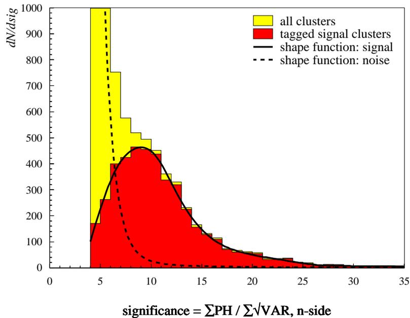
Figure 4.8: *Shape functions for separating signal- and noise clusters. Light histogram: all clusters on half-ladders crossed by a track, dark histogram: tagged signal clusters, solid curve: shape function  $S_{signal}(sig)$  for signal clusters, dashed curve: shape function  $S_{noise}(sig)$  for noise clusters*
