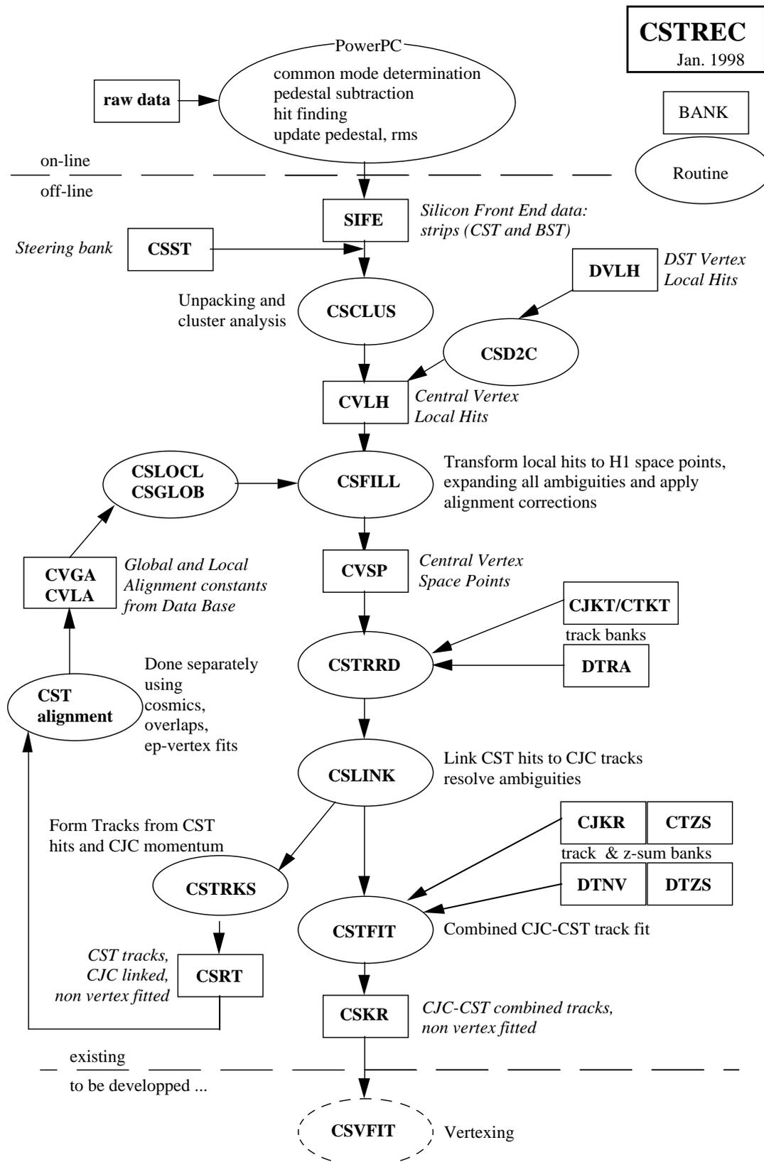
Figure 4.1: Flow diagram of the CSTREC reconstruction module
