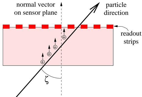
Figure 4.6: Schematic drawing of the dependence of the number of strips carrying signal charge on the incidence angle  $\zeta$  of the particle on the silicon sensor
