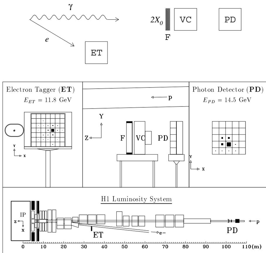
Figure 2.6: *Luminosity detectors and principle of the measurement. The electron radiates a photon which is measured in the photon detector (PD) after having traversed the lead filter (F) and the Čerenkov-counter (VC).*
