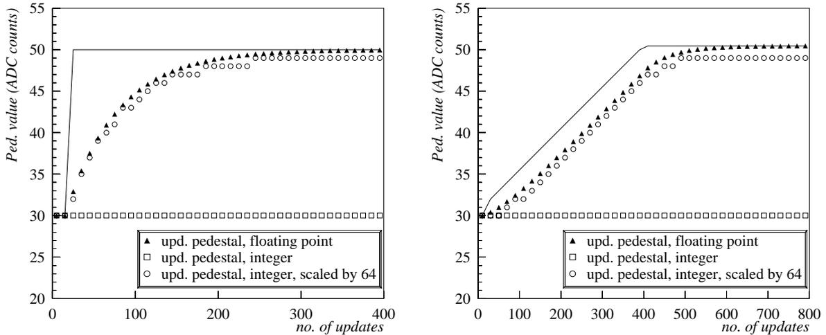
Figure 3.5: Simulated pedestal behaviour with different data types. The line simulates the evolution of the “real” pedestal: a sudden jump of 66% (left) and a steady rise (right). The open circles show the updated values as produced by the implemented algorithm.
