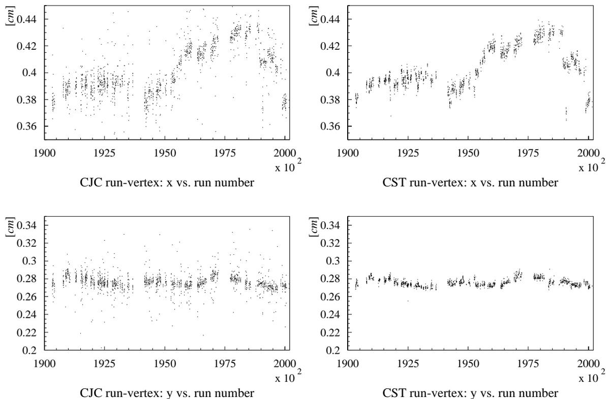
Figure 4.23: *Distribution of the  $x$ - and  $y$ -coordinates of the run vertex for the data taking period 1997 determined by the CJC (left) and with CST tracks (right)*
