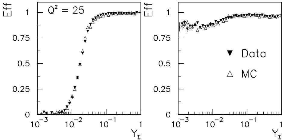
Figure 6.3: Vertex reconstruction efficiency as a function of  $y_\Sigma$  for  $Q^2 = 25 \text{ GeV}^2$ . For the left plot only central tracker vertices are used, the right plot is based on both CIP or the central tracker vertices.
