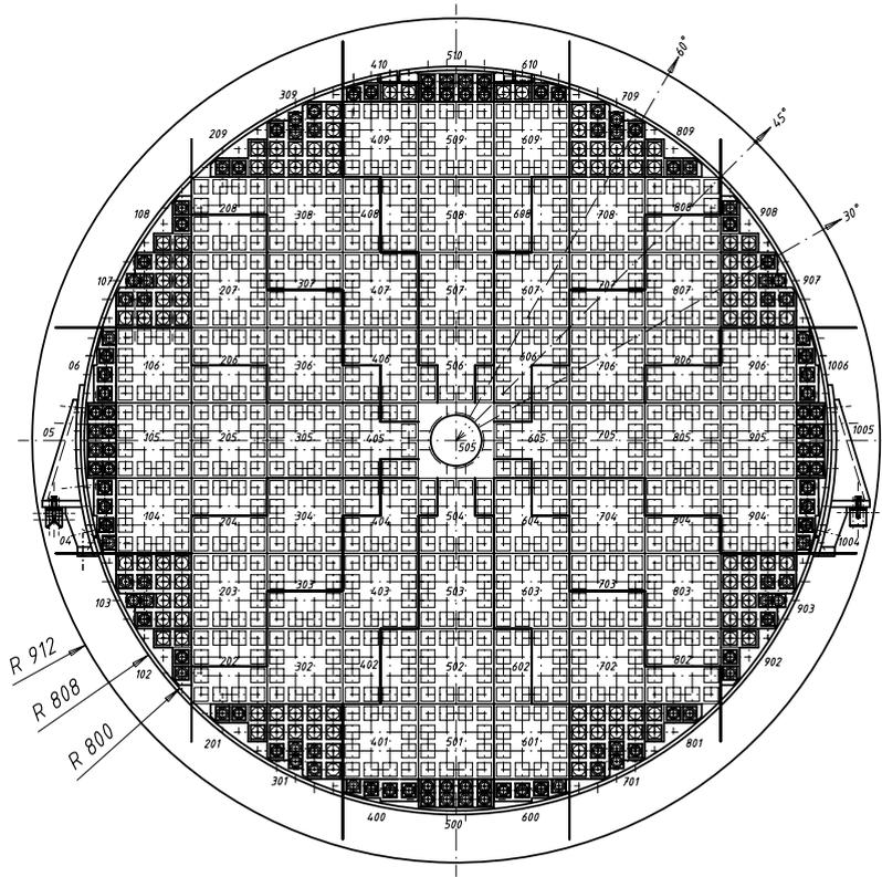
Figure 2.5: Transverse view of the Spacal. Small boxes indicate individual cells. They are combined in  $4 \times 4$  groups into super-modules.
