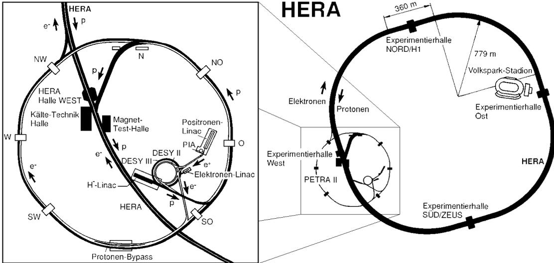
Figure 2.1: Schematic view of the  $ep$  storage ring HERA (right) together with the major experiments. The left figure presents a zoomed view of the HERA preaccelerator chain.
