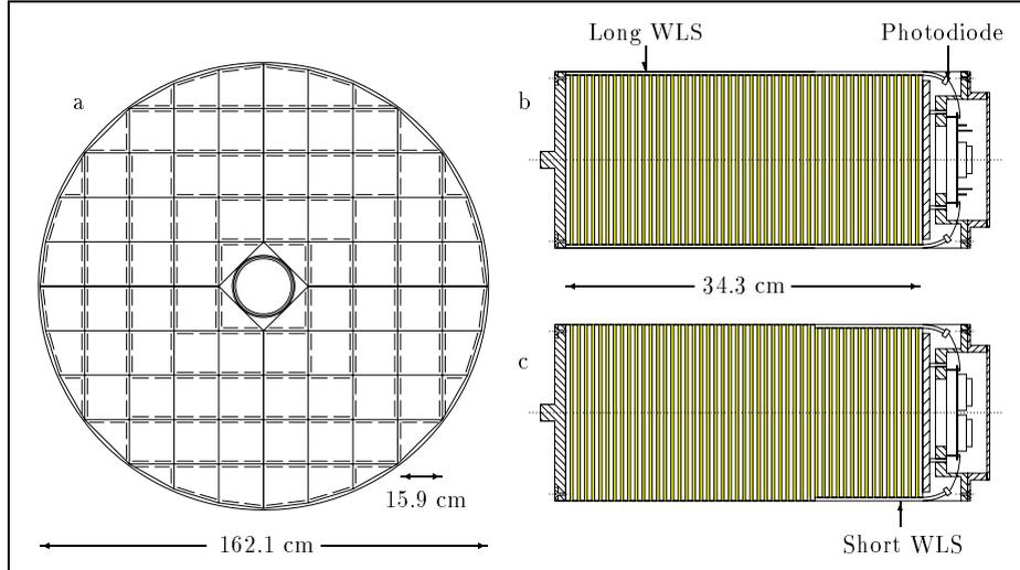
Figure 2.4: a) Transverse view of the backward electromagnetic calorimeter (BEMC). b,c) Longitudinal views of BEMC stacks in two perpendicular planes. The orientation of long wavelength shifters is indicated by horizontal and vertical lines. (from [47])
