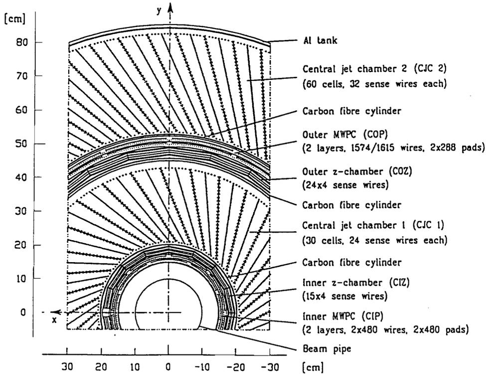
Figure 2.3: Radial view of the H1 central tracker
