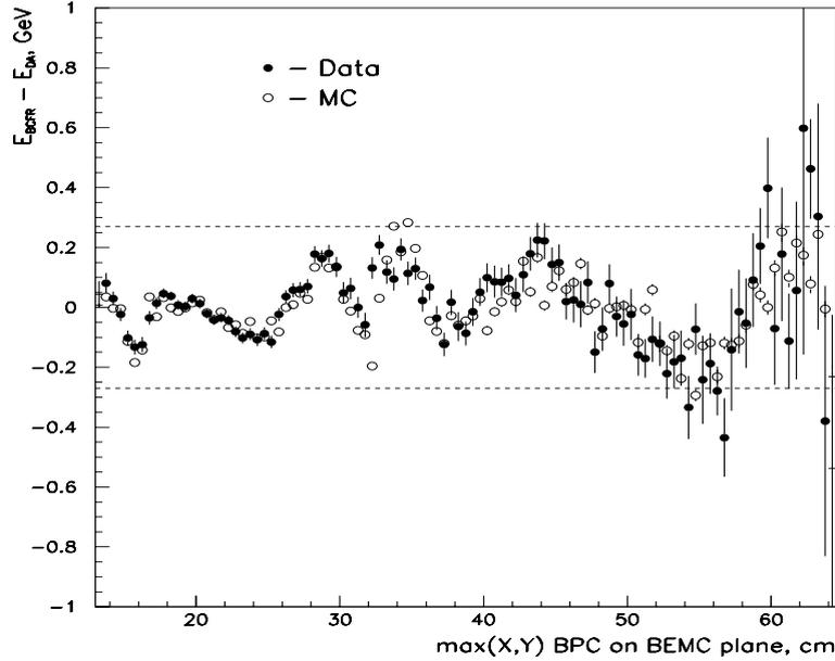
Figure 5.8: Comparison of the BEMC energy calibration for data and Monte Carlo simulation using the double angle method. The difference  $E_{BEMC} - E_{DA}$  is shown as a function of the maximum of the  $|X|$  and  $|Y|$  coordinates of the electron impact point. The dashed lines indicate deviations of  $\pm 1\%$ .
