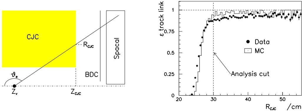
Figure 6.14: Left: schematic view of the  $R - Z$  cross section of the backward H1 detector, used for the CJC link efficiency definition. Right: CJC track link efficiency as a function of  $R_{CJC}$  for data and Monte Carlo simulation.
