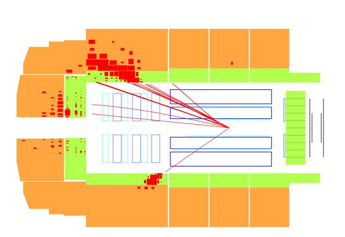
Energy flow algorithm (HFS) combines information from tracker and calorimeters
