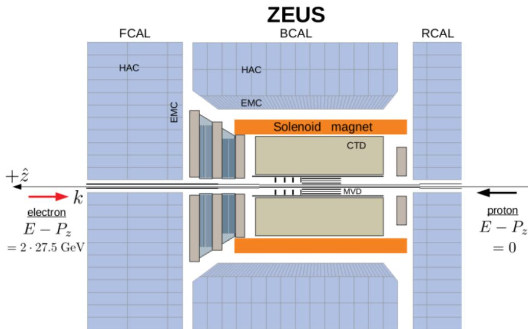
Charged particles are tracked in the central tracking detector (CTD) and micro vertex detector (MVD) in a 1.43 T magnetic field.
