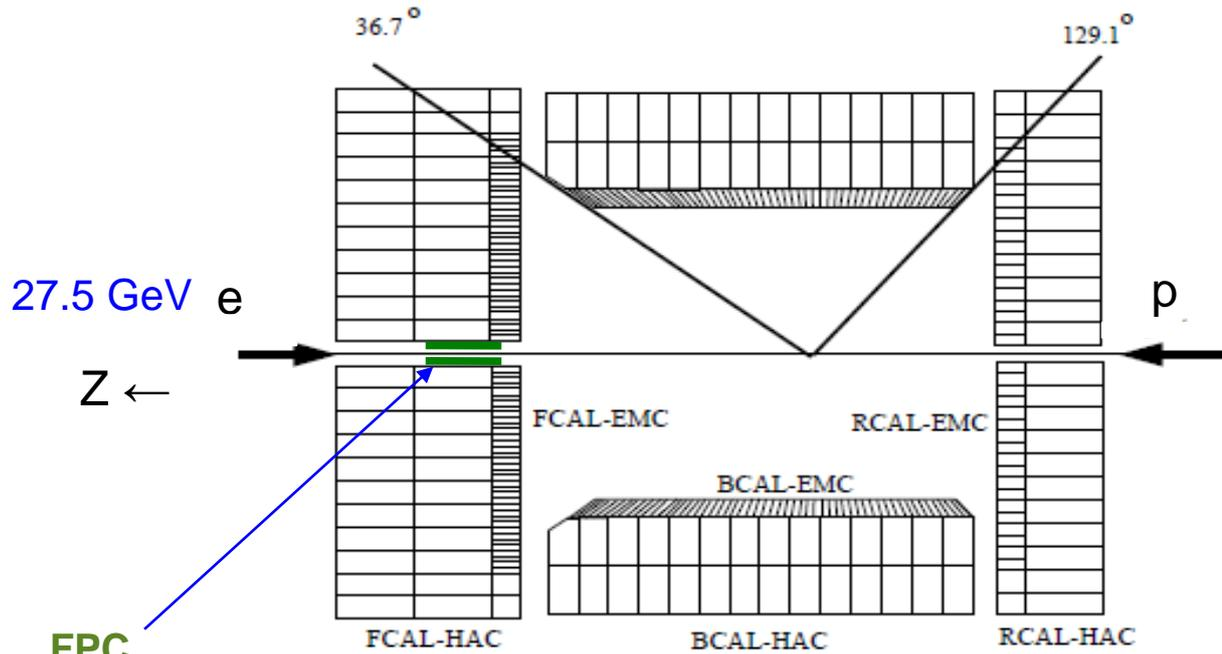
Hard scattered photons are measured in the BCAL, which is finely segmented in the Z direction.
