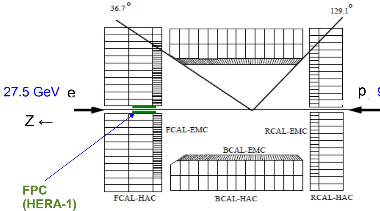
Hard scattered photons are measured in the BCAL, which is finely segmented in the Z direction.
