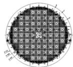
SpaCal is lead/scintillator-fiber calorimeter, backward in H1
