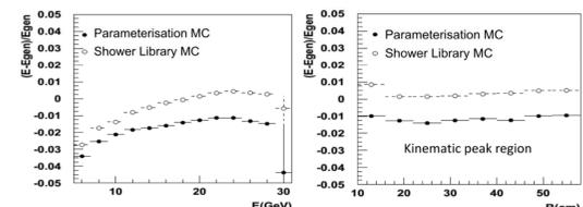
As expected energy resolution deteriorates for lower energies when background contribution (mainly from hadrons) is larger
