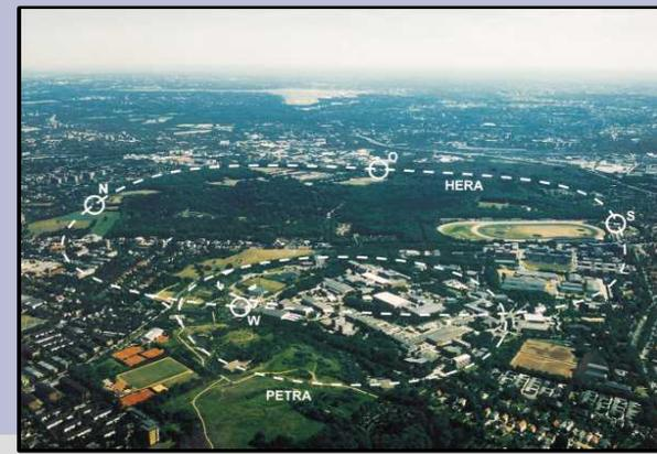
Hera is a 6 km long accelerator located in Hamburg. It collides  $p^+$  at 920 GeV with  $e^\pm$  at 27.5 GeV.
