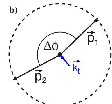
Gluon radiation or initial parton  $k_t$  can lead to non back to back topologies
