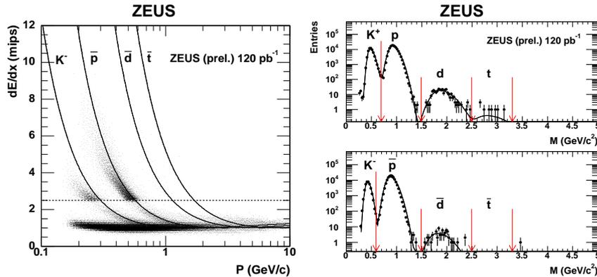
Figure 1. (Left) The  $dE/dx$  distributions as a function of the track momentum for negative charged tracks. The DIS events were accepted by requiring at least one track with  $dE/dx > 2.5$  mips. The curves show the mean energy loss derived using the Bethe-Bloch equation for different particle species. (Right) The mass spectra for positive and negative charged particles. Tracks are selected with  $dE/dx > 2.5$  mips. The arrows show the cuts for each particle species.
