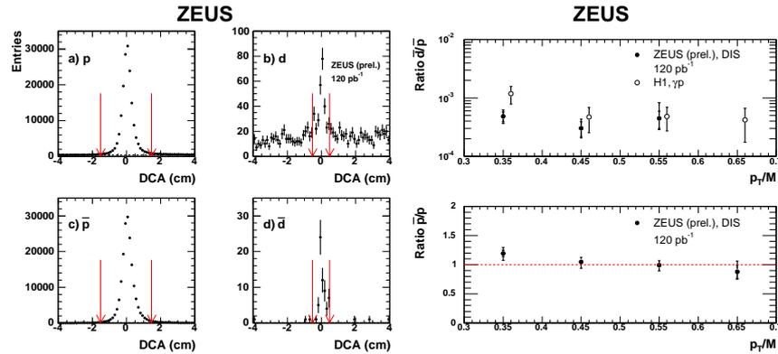
Figure 2. (Left) The distributions of the distance of closest approach for different particle species. The arrows show the signal region. (Right) The top plot shows the corrected  $\bar{d}/\bar{p}$  production ratios as a function of  $p_T/M$ . The measurements are compared to the H1 photoproduction results. The bottom plot shows the  $\bar{p}/p$  ratios.
