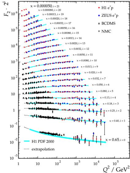
Figure 1.  $F_2$  values measured by H1, ZEUS and fixed target experiments as functions of  $Q^2$  at different  $x$  values. The bands represent the H1 PDF 2000 fit performed to the H1 NC and CC data with  $Q^2 > 3.5$  GeV<sup>2</sup>. The dashed lines depict the extrapolation of the fit towards lower  $Q^2$  values.
