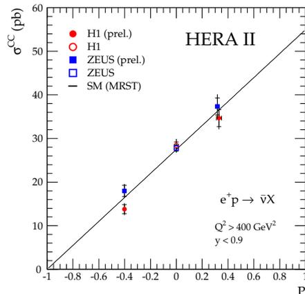
Figure 5. CC cross-sections of  $e^+p$  collisions measured by H1 and ZEUS during the years 2003–2004 of the HERA II data taking period for different  $e^+$ -beam polarizations. The solid line represents the Standard Model prediction involving proton PDF parametrizations by the MRST group.
