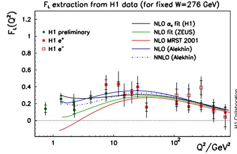
Figure 4.  $F_L$  measurements by H1 for  $W = 276 \text{ GeV}$  and different  $Q^2$  compared to the predictions of pQCD calculations.
