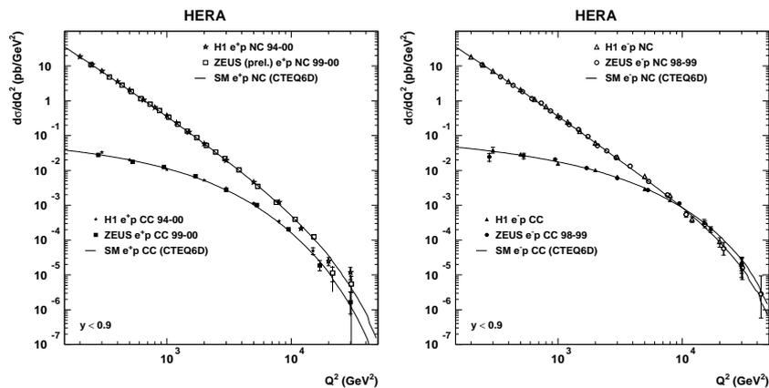
Figure 1. Measurements by H1 and ZEUS of the positron (left) and the electron (right) proton scattering cross sections at large  $Q^2$  in neutral and charged current scattering. The curves represent calculations of the DIS cross section using standard model electroweak couplings and a set of parton distributions determined by the CTEQ Collaboration.
