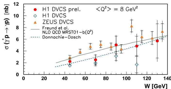
Figure 6. The  $\gamma^*p \rightarrow \gamma p$  DVCS cross section as a function of  $W$  measured by H1 and ZEUS. The data are compared with NLO QCD using a GPD parameterisation (solid curve) and with a Colour Dipole model prediction (dashed curve).
