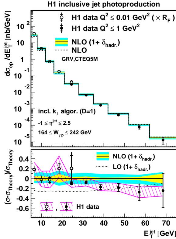
Figure 3. Top: Differential cross section for inclusive jet production as a function of the jet transverse energy. Bottom: relative difference between the data, the LO QCD prediction and the NLO calculation including hadronisation corrections.
