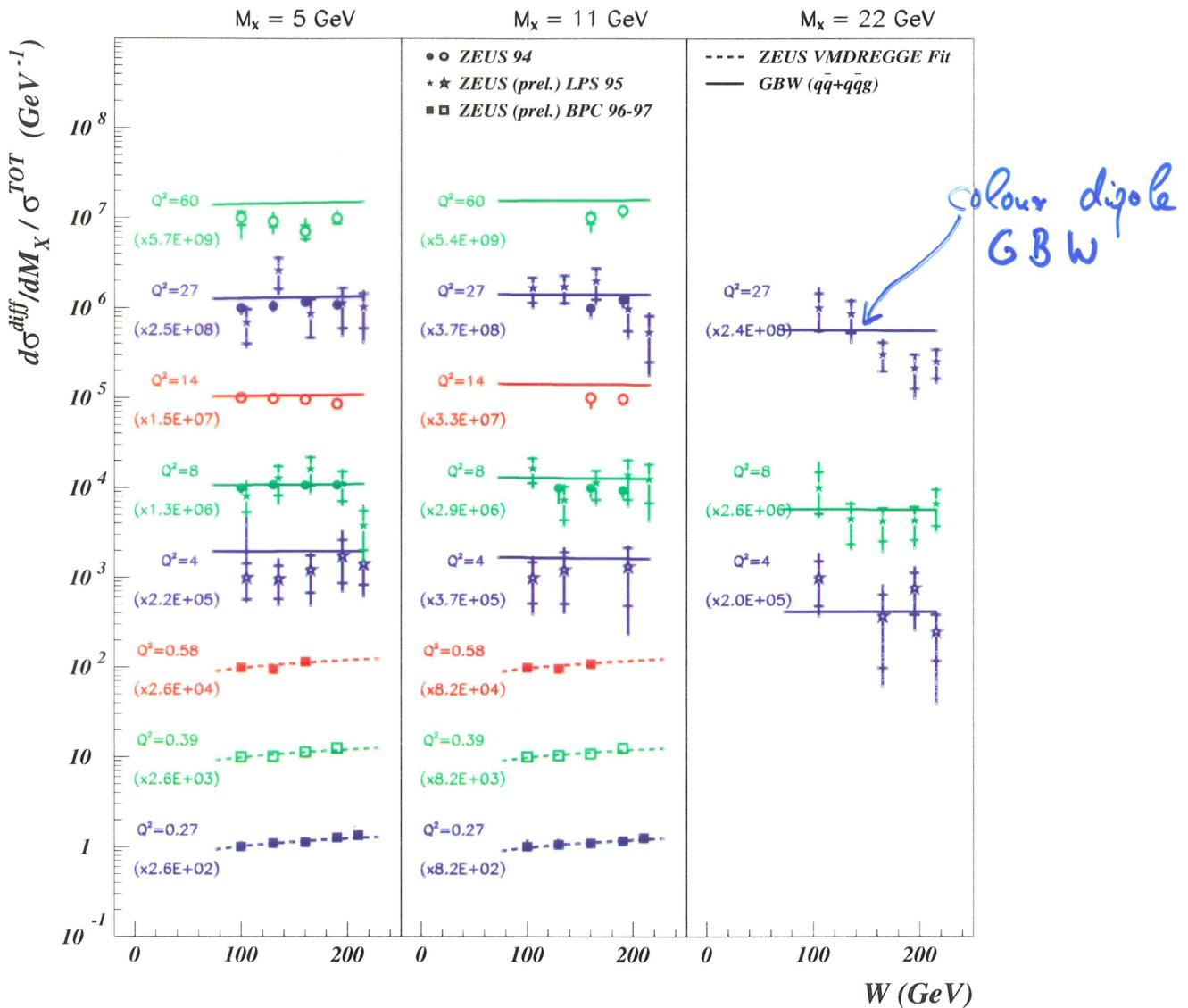
Fits to  $\frac{\int dt \frac{d\sigma_{\gamma^* p \rightarrow XY}^{\text{diff}}}{dM_X} dt}{\sigma_{\gamma^* p \rightarrow X}^{\text{tot}}} \propto W^\rho$
