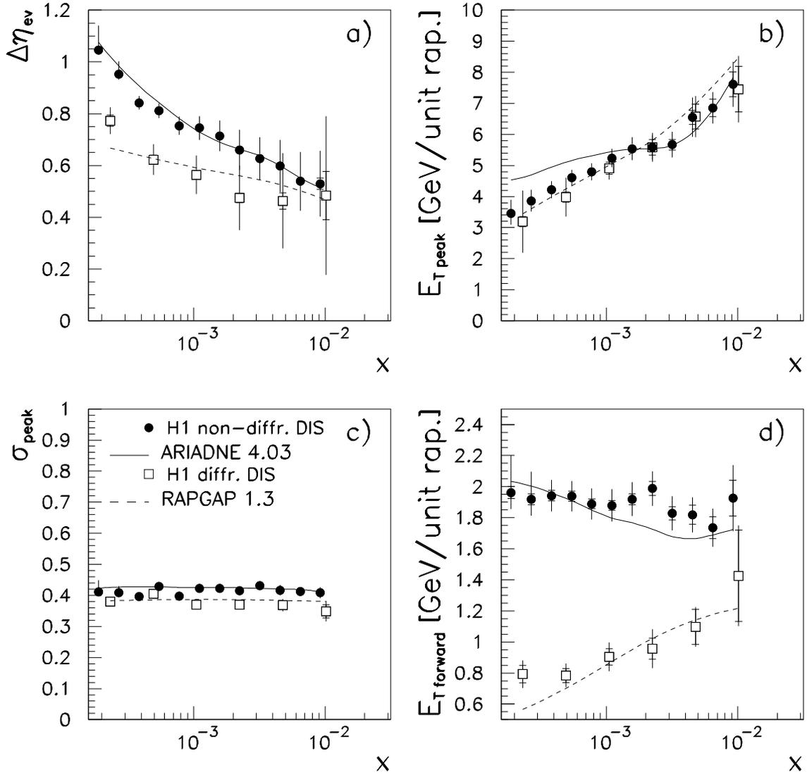
**Figure 3:** Measured estimators of the transverse energy flow for non-diffractive (“non-diffr. DIS”) and diffractive (“diffr. DIS”) DIS, compared with the ARIADNE and RAPGAP models. Shown is the dependence on  $x$  for the measured deviation from the calculated direction (a), for the magnitude of the current region (b), for the width of the current region (c) and for the forward transverse energy (d).
