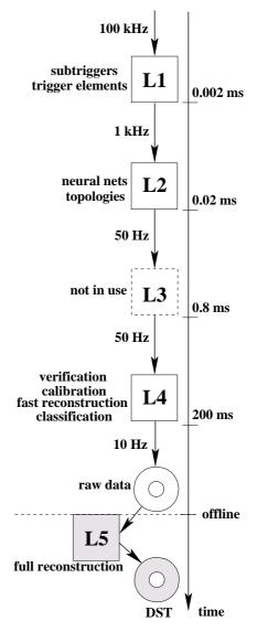
Figure 2.6: The H1 Trigger System.
