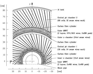
Figure 2.3: The (x, y) plane wire structure of the CJC.
