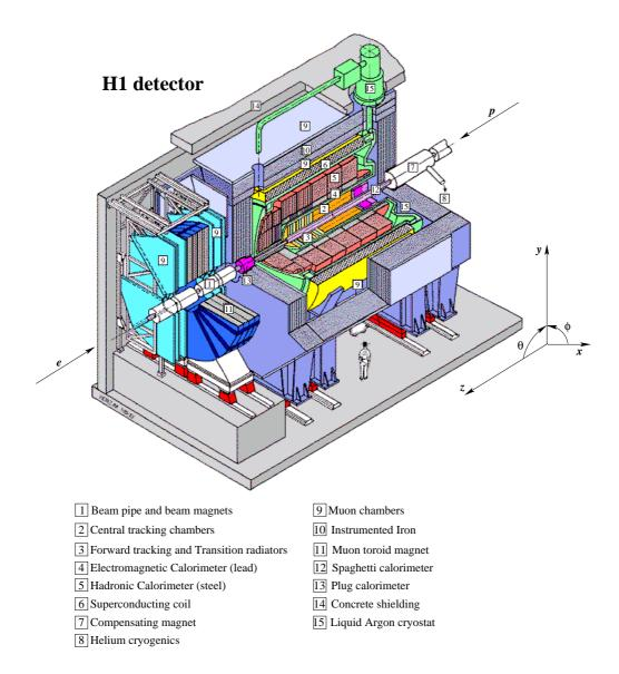
Figure 2.2: The H1 detector architecture.
