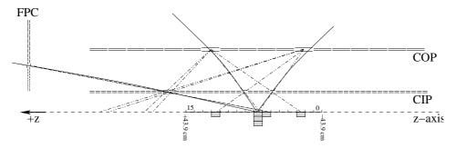
Figure 3.3: Sketch of the online determination of the **zVtx\_sig** trigger element.
