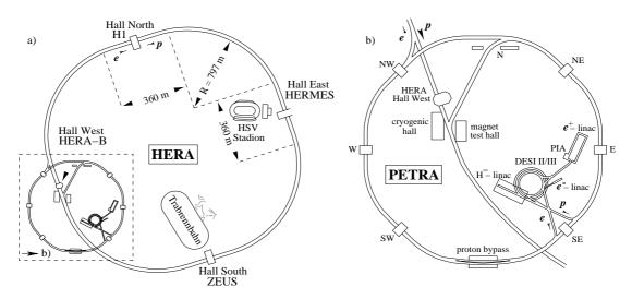
Figure 2.1: The geometry of the HERA collider a) and its pre-accelerators b).
