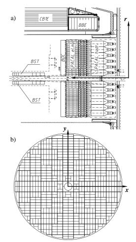
Figure 2.5: The SpaCal; a) longitudinal and b) transversal section.
