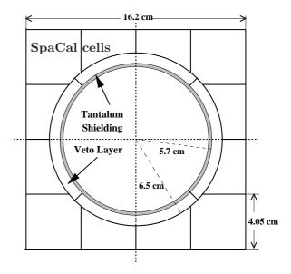
Figure 3.14: The (x, y) view of the SpaCal inner cells and the VETO layer.
