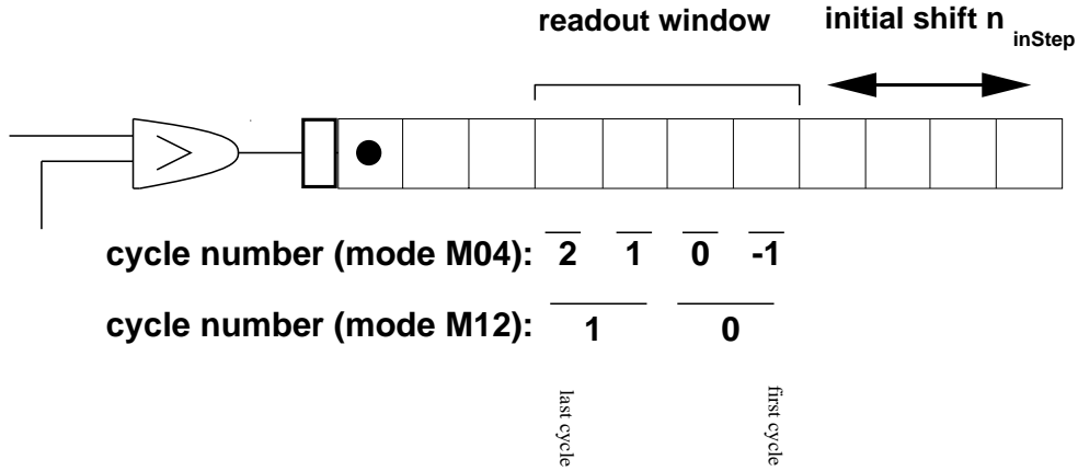
Figure 6.1.: The correspondence between readout cycle numbers and pipeline positions for different modes of operation (see section 4.2.1).
