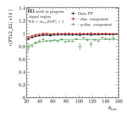
Figure 6.13: Efficiency of the FTi2 veto as a function of the lower track angle  $\theta_{\text{low}}$ . The efficiency is measured in the subsample of the photoproduction dataset that was recorded without the FTi2 veto in the online trigger definition. The efficiency is separated for elastic and proton-dissociative events as described in the text and as labeled in the legend. Only statistical uncertainties are considered.
