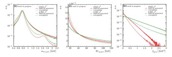
**Figure 5.2:** Generated and tuned lineshapes for the elastic and proton-dissociative DiffVM  $\rho^0$  MC sample as a function of  $m_{\pi\pi}$  (left),  $W_{\gamma p}$  (center), and t (right).
