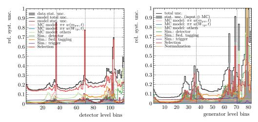
Figure 7.10: Uncertainty breakdown for the one-dimensional  $m_{\pi\pi}$  distributions before (left) and after unfolding (right). The impact of various sources of Uncertainties as labeled in the legends is compared.
