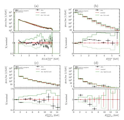
Figure 5.5: Impact of the LAr and SpaCal energy scale variations of the respective total energy deposits for events satisfying the base selection. (a) SpaCal energy associated to the tracks, (b) SpaCal energy not associated to the tracks, (c) LAr energy associated to the tracks, and (d) LAr energy not associated to the tracks. The black data points are compared to the nominal and varied MC samples as labeled by the legend.
