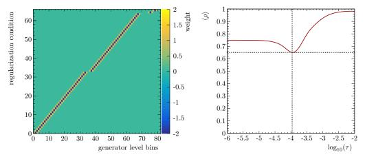
Figure 7.8: Regularization matrix L for the unfolding of the one-dimensional  $m_{\pi\pi}$  distributions (left) and scan of the average global correlation coefficient  $\langle \rho \rangle$  over the regularization strength  $\tau$  (right). For the actual unfolding  $\tau$  is chosen to minimize  $\langle \rho \rangle$  as is indicated by the dashed lines.
