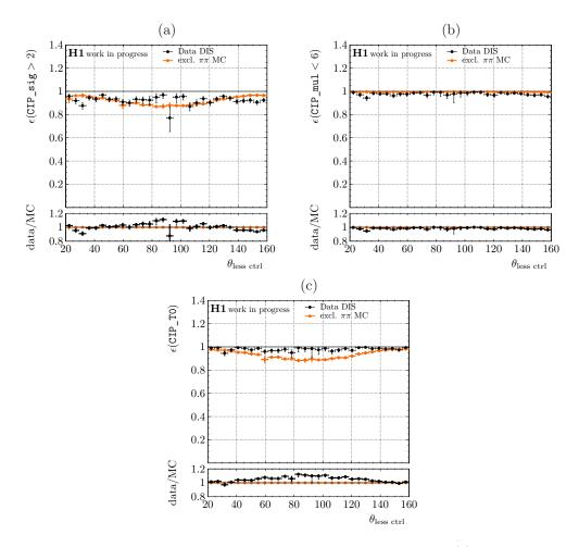
**Figure 6.8:** Efficiency of the CIP s14 trigger elements CIP\_sig>2 (a), CIP\_mul<6 (b), and CIP\_T0 (c) as a function of  $\theta_{less\ ctrl}$ . The efficiencies are measured in the DIS data sample and compared to the corresponding MC model. Only statistical uncertainties are considered.
