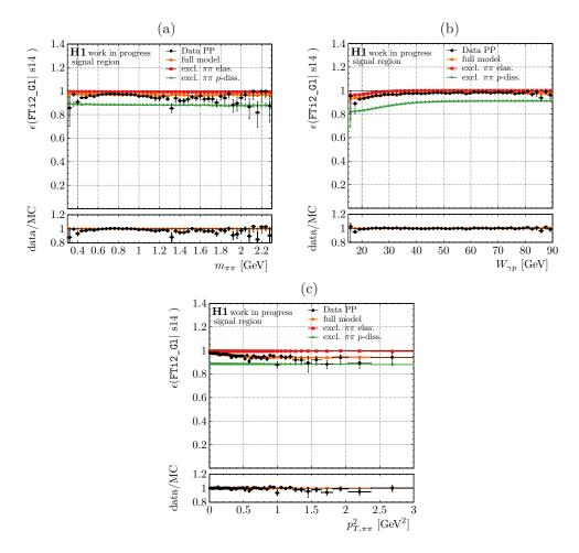
Figure 6.14: FTi2\_G1 veto efficiency in the photoproduction data subsample as a function of  $m_{\pi\pi}$  (a),  $W_{\gamma p}$  (b), and  $p_{T,\pi\pi}^2$  (c) after applying the trigger correction to the elastic and proton-dissociative MC samples. The black data points are compared to the full MC model and the elastic and proton-dissociative  $\pi^+\pi^-$  signal samples as labeled in the legend. Only statistical uncertainties are considered.
