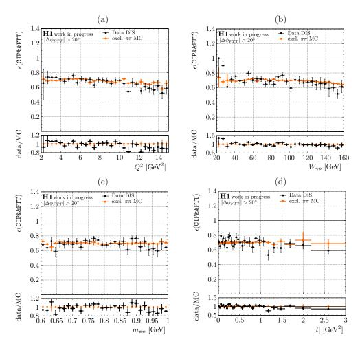
**Figure 6.12:** Efficiency of the combined CIP&&FTT s14 trigger elements measured in the DIS data and MC sample as a function of  $Q^2$  (a),  $W_{\gamma p}$  (b),  $m_{\pi\pi}$  (c), and t (d). The MC efficiency is corrected as described in the text. Only statistical uncertainties are considered.
