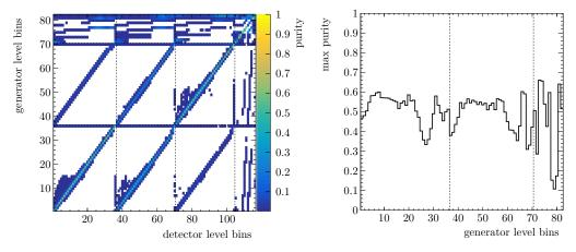
Figure 7.7: Purity matrix (left) and maximum entry for every generator level bin (right) for the one-dimensional  $m_{\pi\pi}$  response matrix. The dashed lines indicate the boundaries of the elastic and proton-dissociative  $\pi^+\pi^-$  signal MC on generator level and the three signal tagging regions on detector level.
