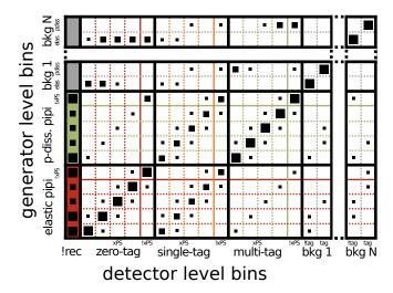
**Figure 7.5:** Illustration of the general structure of the response matrices used for the unfolding. The x-axis corresponds to reconstructed detector level variables, the y-axis to the true, generator level variables.
