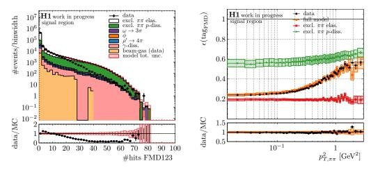
**Figure 4.22:** Left: Distribution of the number of hits in the first three FMD layers. The black data points are compared to the MC model with stacked contributions as labeled in the legend. Right: FMD tagging rate as a function of  $p_{T,\pi\pi}^2$ . The rate is shown for data, the full model, and the elastic and proton-dissociative signal MC as labeled in the legend.
