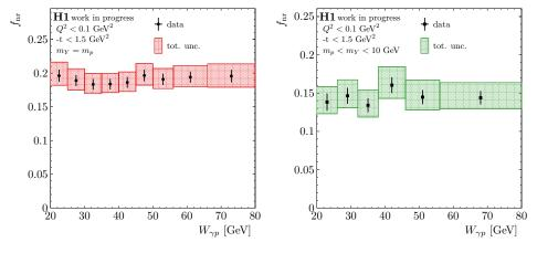
**Figure 8.4:** Fit parameters  $f_{\rm nr}$  as a function of  $W_{\gamma p}$ . The parameters are obtained from the Söding fit to the double-differential cross-sections  $d\sigma(\gamma p \to \pi^+\pi^- Y)/dm_{\pi\pi}(m_{\pi\pi}, W_{\gamma p})$  that is described in the text. The left and right plot show the elastic and proton-dissociative parameter values, respectively.
