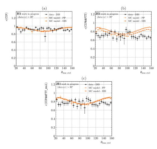
**Figure 6.10:** Efficiencies  $\epsilon_{\text{CIP}}$  (a),  $\epsilon_{\text{CIP&&FTT}}$  (b),  $\epsilon_{\text{CIP&&FTT}_{mul}}$  (c) as a function of  $\theta_{\text{less ctrl}}$ . The efficiencies are measured in the DIS data sample and in the DIS and photoproduction MC samples as labeled in the legend. Only statistical uncertainties are considered.
