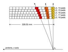
Figure 3.4: Projective geometry of the CIP. Tracks originating from the same position along the z-axis create the same hit pattern. The pattern is shifted along the z-axis by a constant number of pads depending on the track  $\theta$ . Figure from Urban [147] and adapted.
