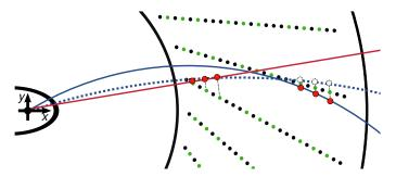
**Figure 6.5:** Illustration of the reconstruction of a fake FTT track. Shown is an drawing of the inner CJC with the sense wires used by the three inner FTT trigger groups marked in green. The fake track (dashed line) is reconstructed from a combination of a real (red dots) and a mirror charge triplet (white dots) that are produced by two real, proximate tracks (continuous lines). The event resembles an actual DIS  $\pi^+\pi^-$  data event.
