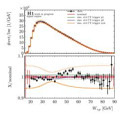
**Figure 5.6:** Uncertainties for the CIP && FTT trigger elements correction as a function of  $W_{\gamma p}$  for events in the  $\pi^+\pi^-$  signal region. The black data points are compared to the nominal and varied MC samples as labeled by the legend.
