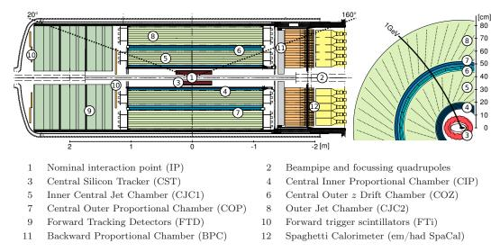
Figure 3.3: Left: Inner part of the H1 detector. Right: Transverse view of one quadrant of the CTD. Images provided by the H1 collaboration and modified.
