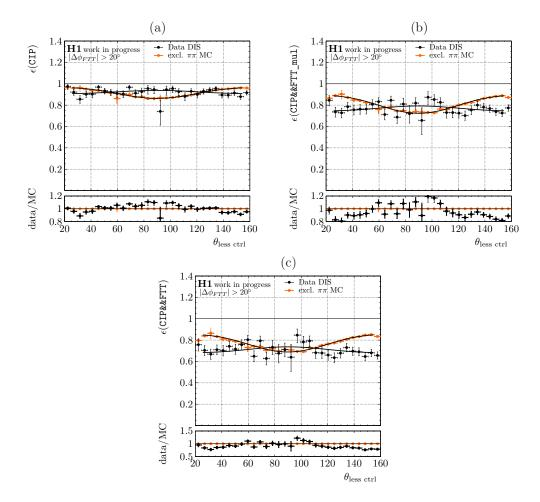
**Figure 6.11:** Fits of the  $\theta_{\text{less ctrl}}$  dependence of the efficiencies  $\epsilon_{\text{CIP}}$  (a),  $\epsilon_{\text{CIP&&FTT}}$  (b),  $\epsilon_{\text{CIP&&FTT\_mul}}$  (c) measured in the DIS data and MC samples. Only statistical uncertainties are considered.
