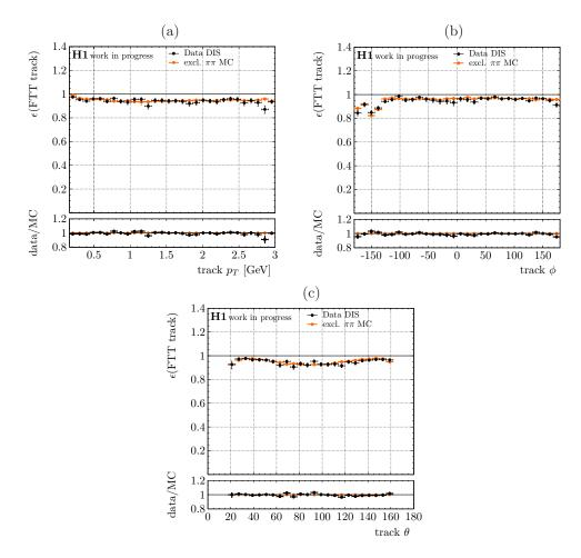
**Figure 6.4:** FTT single track reconstruction efficiency measured in DIS as a function of the offline reconstructed track  $p_T$  (a),  $\phi$  (b), and  $\theta$  (c). Only statistical uncertainties are considered.
