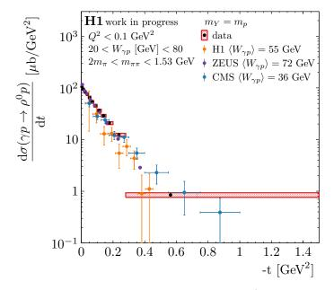
**Figure 8.10:** Differential elastic cross-section  $d\sigma(\gamma p \to \rho^0 p)/dt$  as a function of t. The measurement presented in this thesis is compared to selected measurements by the H1 [6], ZEUS [11], and CMS [195] Collaboration at comparable center-of-mass energies.
