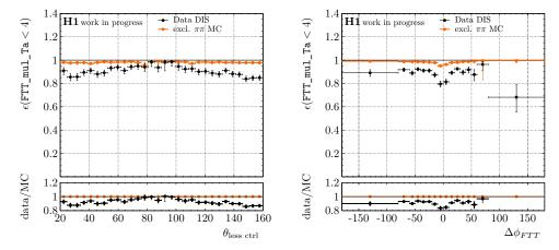
Figure 6.6: FTT\_mul\_Ta<4 efficiency in DIS as a function of the azimuthal opening angle between the two tracks evaluated at the radius of the third FTT layer  $\Delta\phi_{\rm FTT}$  (left), and as a function of the less central track angle  $\theta_{\rm less\ ctrl}$  (right). Only statistical uncertainties are considered.
