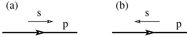
Figure 2.4: Helicity is the projection of spin along the direction of motion \vec{s} \cdot \vec{p}/|\vec{s}| \cdot |\vec{p}| . A particle with spin parallel (helicity +1 ) and antiparallel (helicity -1 ) to the direction of motion is called right-handed (a) and left-handed (b), respectively.
