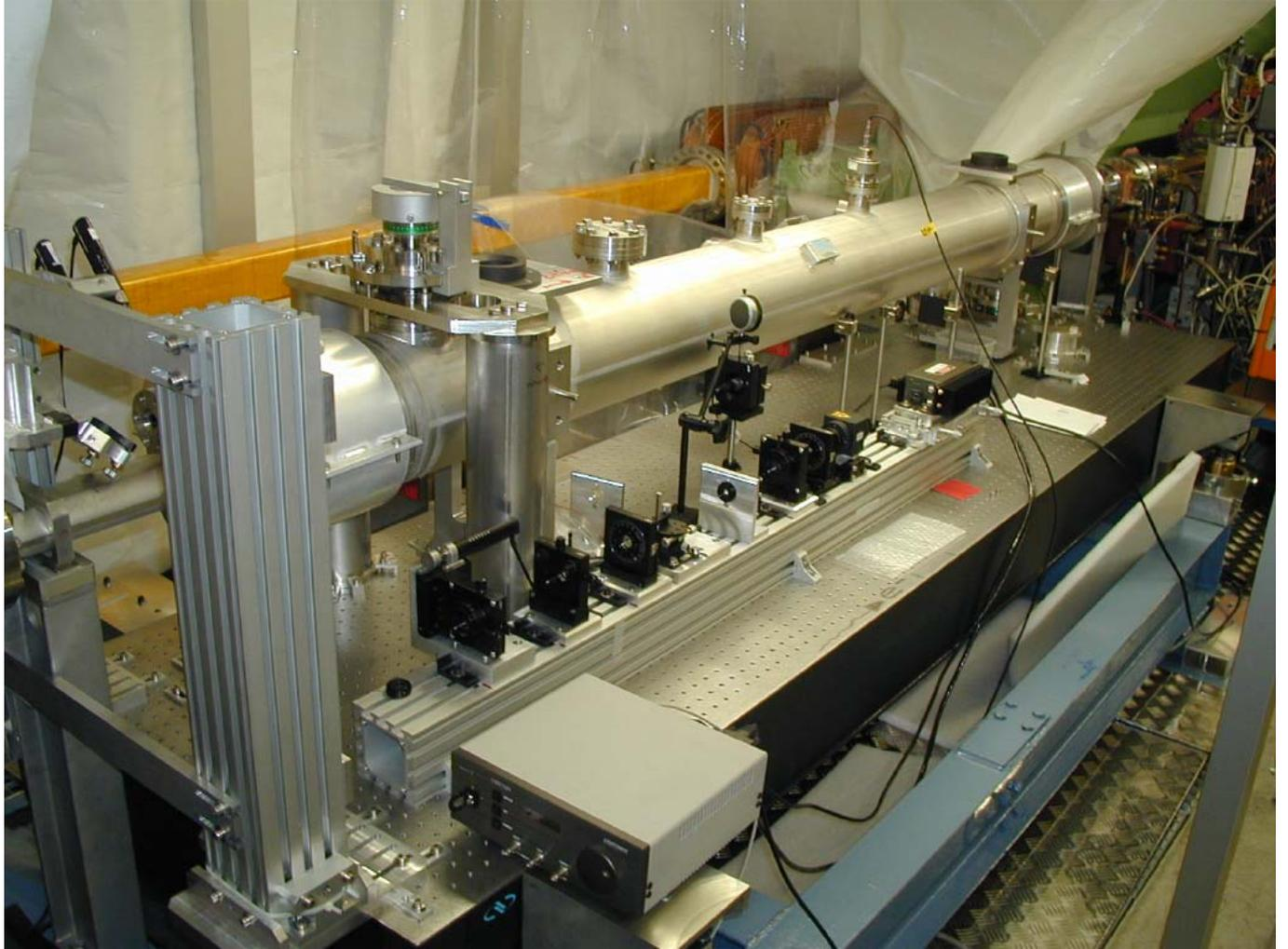
Figure 3.7: *Picture of the cavity taken during the installation. The laser and the optical elements before the cavity entrance are located on the rail parallel to the cavity vessel. The red laser diode, used to aligned the cavity mirrors, enters the cavity by the opposite entrance. It is visible on the picture: between the rail and the cavity vessel and mounted on a post holder at a height higher than the rail.*
