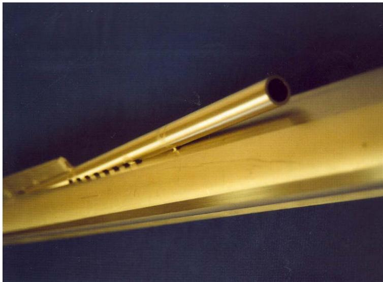
Figure 3.5: *Picture of beam pipe inside the cavity (half is shown). Above the elliptic electron beam-pipe, a circular tube is soldered to reduce the wakefield excitations.*
