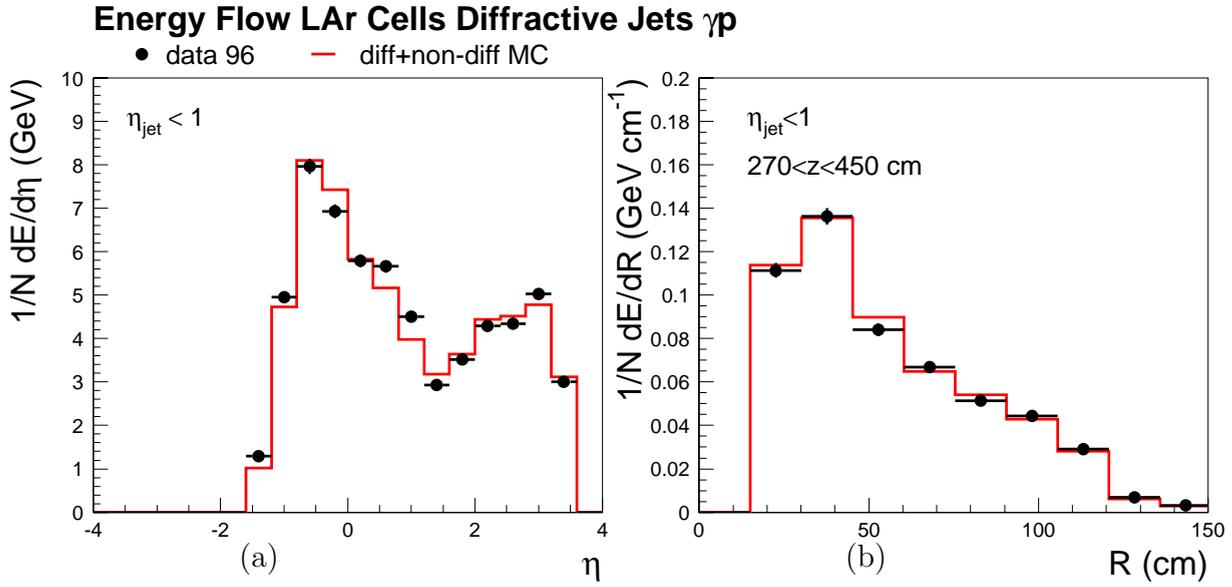
**Fig. 5.18.** Average LAr calorimeter cell energy in dijet events with  $x_P < 0.03$  and  $\sum_{1:3} \text{FMD} < 2$  for 96. The energy is shown as a function of (a) the pseudorapidity  $\eta$  in the laboratory frame, and (b) the radial distance  $R$  from the beam axis for the forward part of the LAr calorimeter ( $270 < z < 450$  cm). The jets are required to satisfy  $\eta_{\text{jet}} < 1$ .
