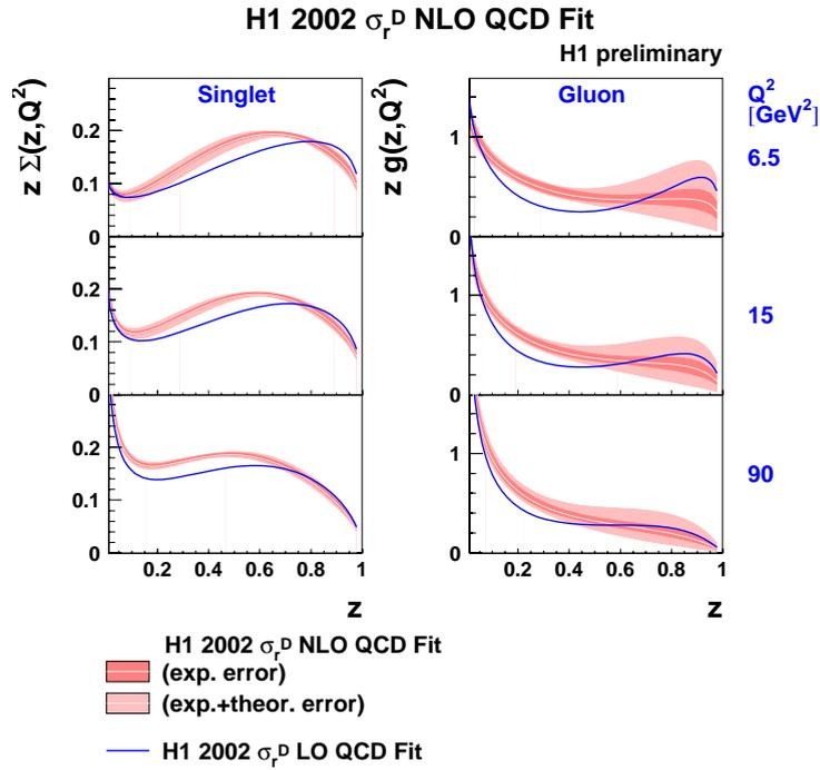
**Fig. 2.3.** Parton distributions of the pomeron at the LO and at the NLO as determined in DGLAP fits to H1  $F_2^D$  data. They are shown as a function of the parton momentum fraction  $z$  at different scales  $Q^2$ . The left plots show the quark distributions, the right plots show the gluon (from [3]).
