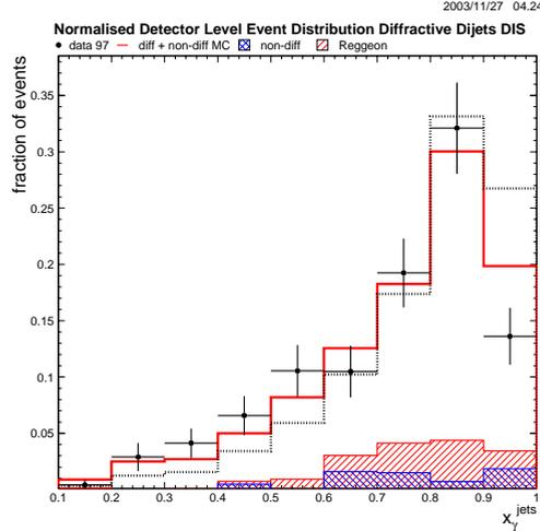
**Fig. 6.18.** The distribution of  $x_\gamma$  for the diffractive DIS dijet sample of 97. The model is reweighted in  $x_\gamma$ . The prediction without the reweight is shown as the dotted histogram.
