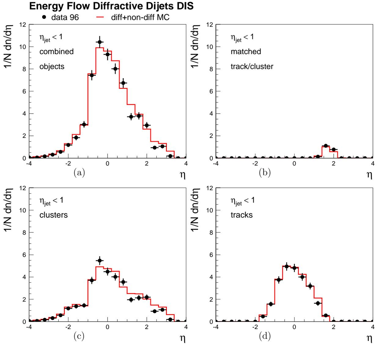
**Fig. 6.20.** Multiplicity for the diffractive DIS dijet sample in 96. Shown is as a function of the pseudorapidity  $\eta$  in the laboratory frame the average number of (a) combined objects from tracks and calorimeter clusters, (b) matched tracks and clusters, (c) clusters, and (d) tracks. The jets are required to satisfy  $\eta_{\text{jet}} < 1$ .
