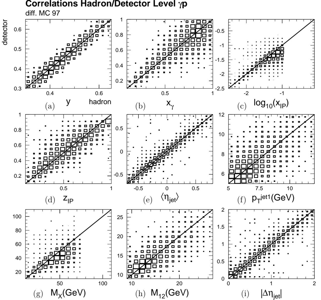
**Fig. 5.1.** Correlations between the variable reconstructed at the hadron level (horizontal axis) and the detector level (vertical axis). The correlations are evaluated with the diffractive MC for 97. All final selection cuts are applied at the detector level and the hadron level except for the distributions of  $\log x_{IP}$  and  $M_X$  for which no diffractive cuts are applied to extend the populated range.
