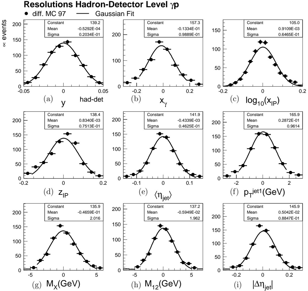
**Fig. 5.2.** Resolutions for reconstructing the hadron level quantity at the detector level. Shown is the difference between the variable reconstructed at the hadron level and at the detector level. The resolutions are evaluated with the diffractive MC for 97.
