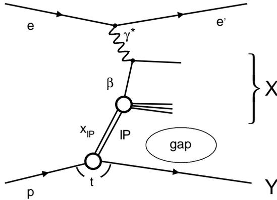
**Fig. 2.1.** Inclusive DDIS process in the resolved pomeron model. The virtual photon scatters off a parton from the pomeron with momentum fraction  $\beta$ . The pomeron ( $IP$ ) carries a fraction  $x_{IP}$  of the proton momentum. A gap is observed between the systems  $X$  and  $Y$ .
