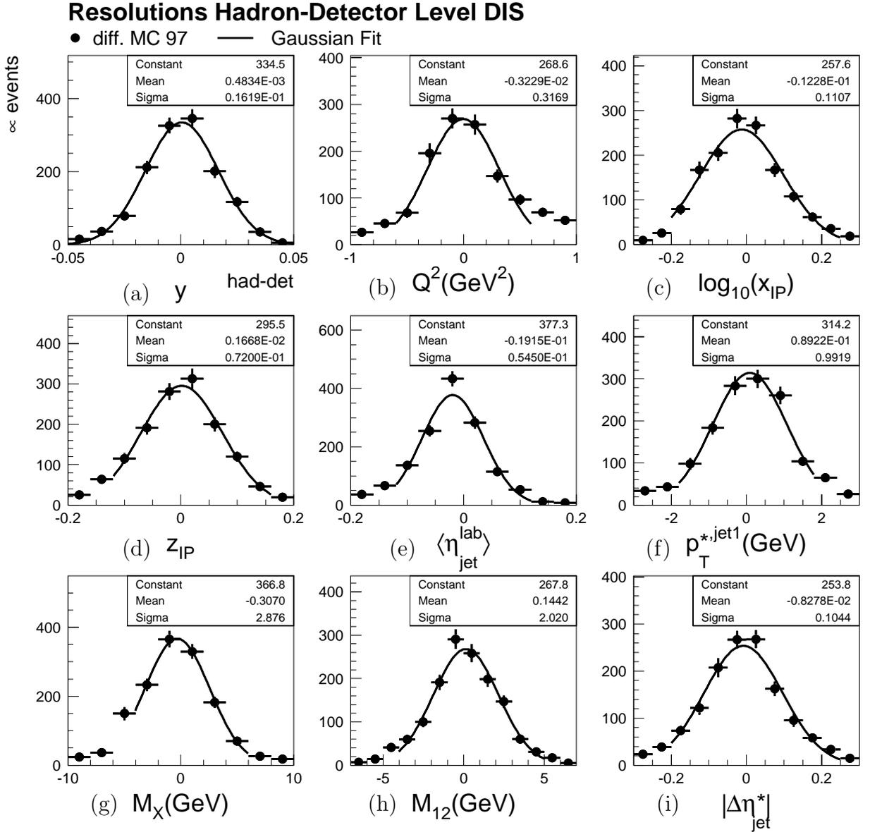
**Fig. 6.2.** Resolutions for reconstructing the hadron level quantity at the detector level. Shown is the difference between the variable reconstructed at the hadron level and at the detector level. The resolutions are evaluated with the diffractive MC for 97.
