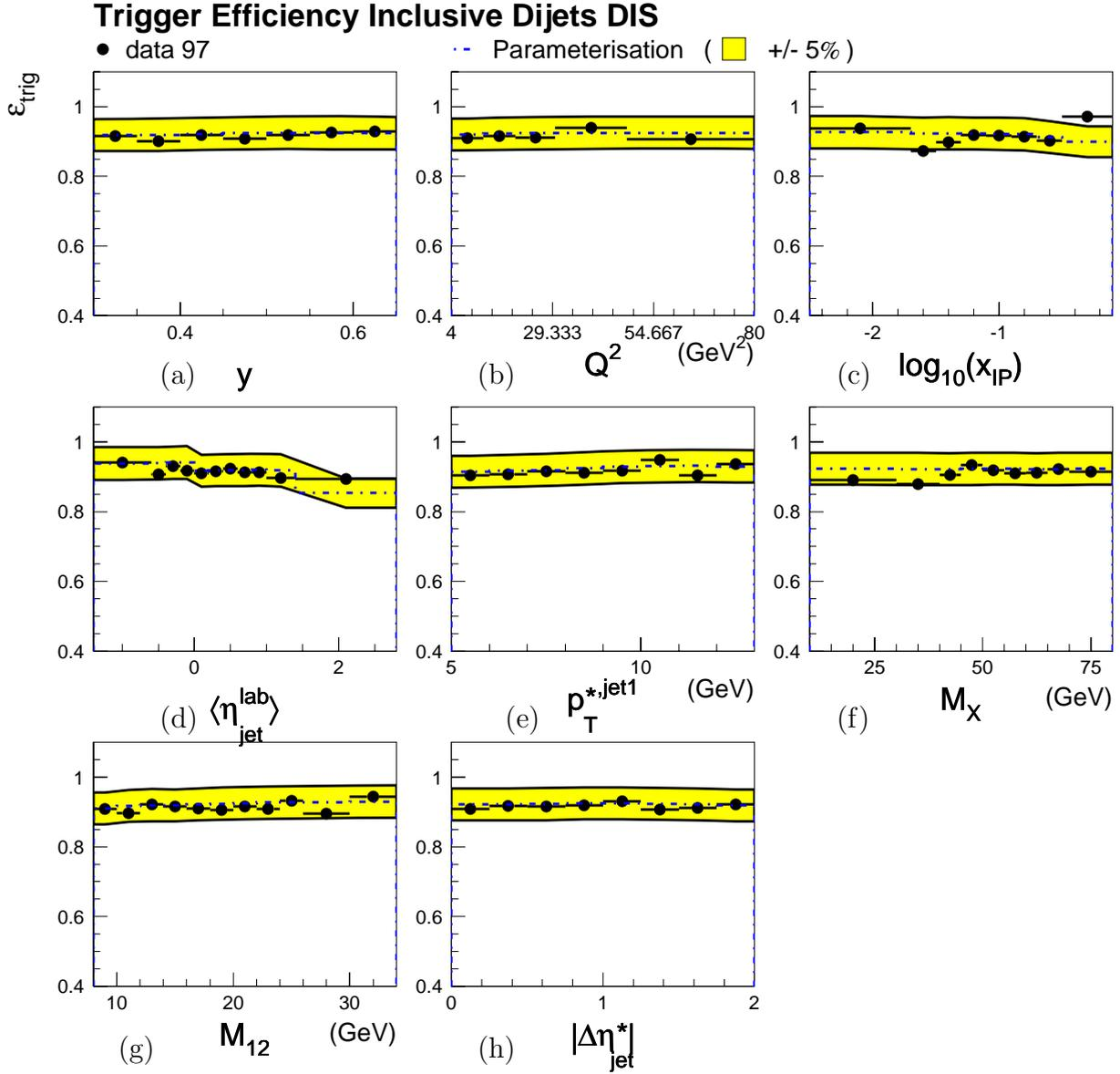
**Fig. 6.8.** Trigger efficiency for inclusive DIS dijets in 97. Also shown as the dotted line is the parameterisation which is used for the correction of the data. A  $\pm 5\%$  band around the parameterisation is indicated which is taken as the uncertainty of the trigger efficiency.
