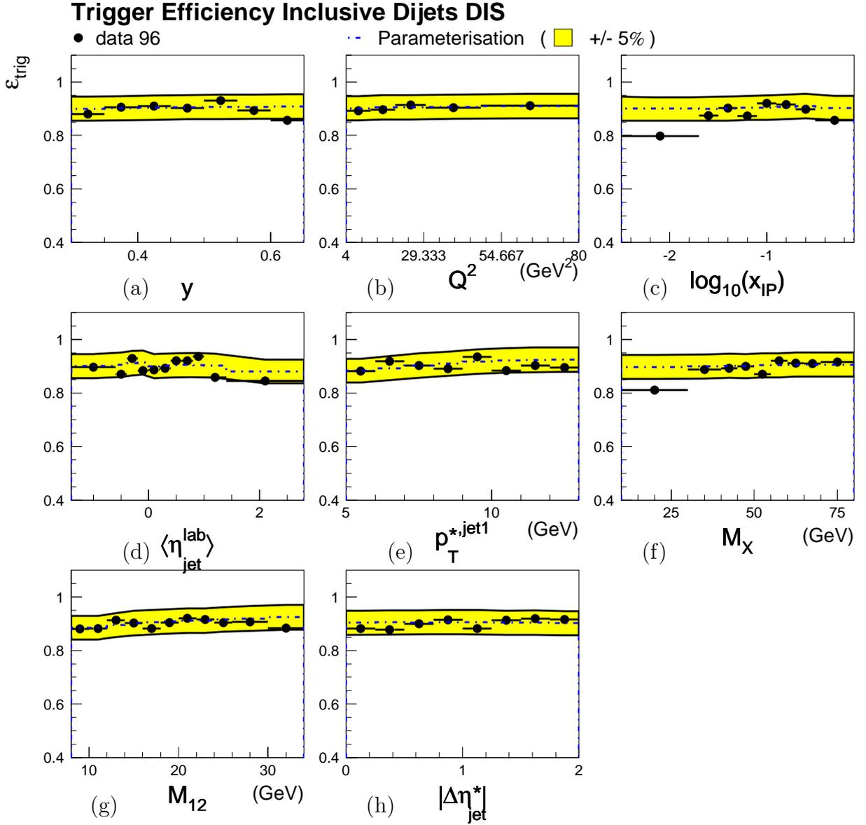
**Fig. 6.7.** Trigger efficiency for inclusive DIS dijets in 96. Also shown as the dotted line is the parameterisation which is used for the correction of the data. A  $\pm 5\%$  band around the parameterisation is indicated which is taken as the uncertainty of the trigger efficiency.
