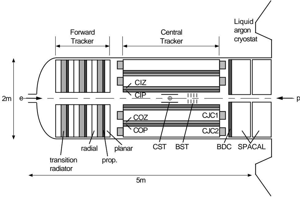
**Fig. 3.4.** The tracking system of the H1 detector.
