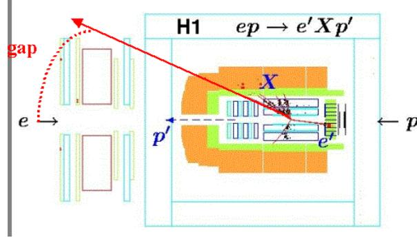
**Fig. 2.2.** An inclusive DDIS event in the H1 detector. The scattered electron is detected, whereas the scattered proton system  $p'$  escapes through the beam pipe. Between the centrally produced system  $X$  and  $p'$  no signals are detected (rapidity gap).
