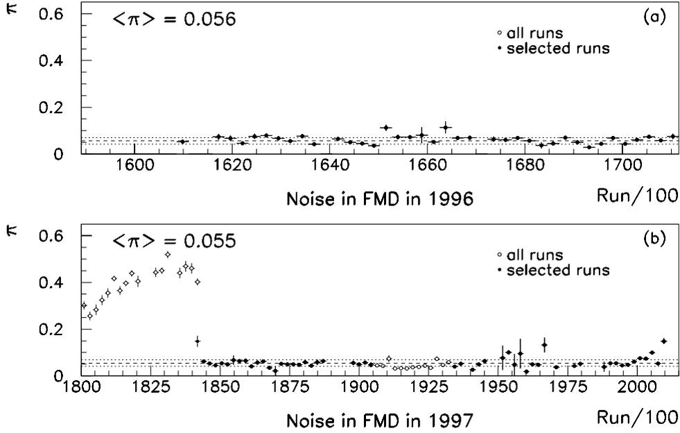
**Fig. 5.13.** Noise in the FMD for (a) 96 and (b) 97 as a function of the run number. Shown is the fraction  $\pi$  of random trigger events fulfilling the cuts  $\sum_{1:3} \text{FMD} > 1, \eta_{\text{max}} < 3.2$ . The region at the beginning of 97 is not included in the analysis (from [37]).
