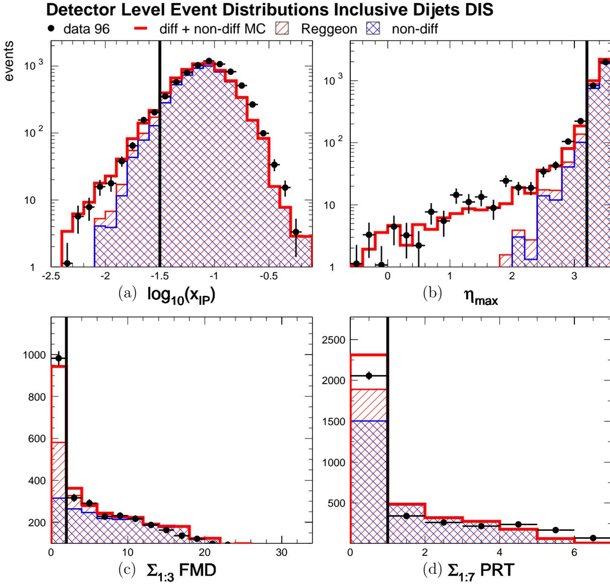
**Fig. 6.14.** Distributions of the diffractive cut variables for the events of the inclusive DIS dijet sample of 96. (a)  $x_{IP}$ , (b)  $\eta_{\max}$ , (c) FMD and (d) PRT. For (c), FMD noise has been added in the MC.
