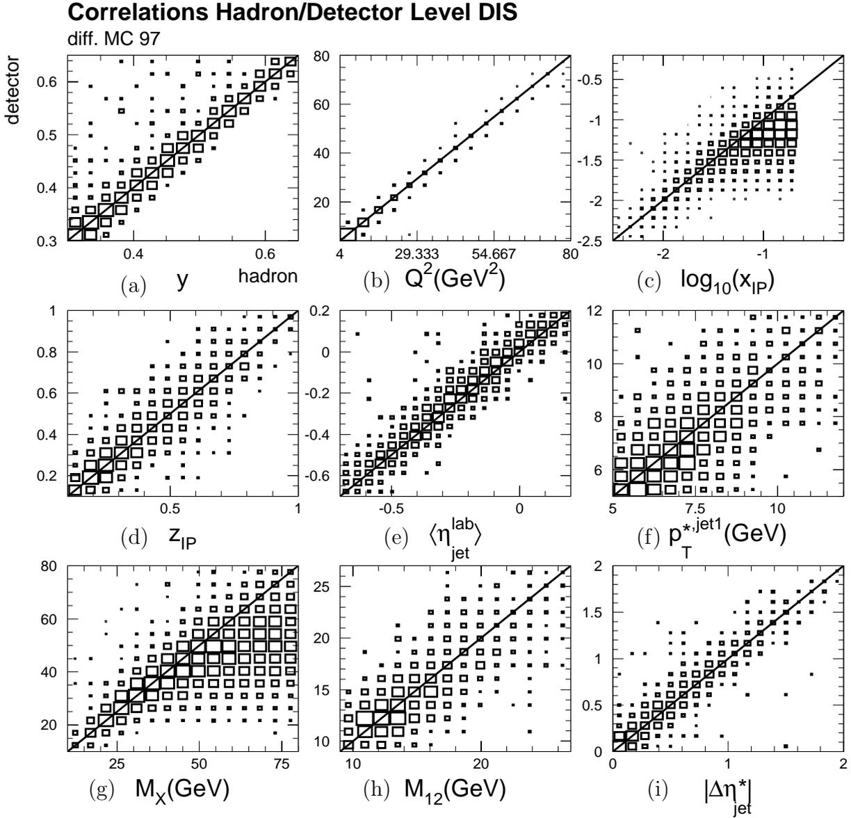
**Fig. 6.1.** Correlations between the variable reconstructed at the hadron level (horizontal axis) and the detector level (vertical axis). The correlations are evaluated with the diffractive MC for 97. All final selection cuts are applied at the detector level and the hadron level except for the distributions of  $\log x_{IP}$  and  $M_X$  for which no diffractive cuts are applied to extend the populated range.
