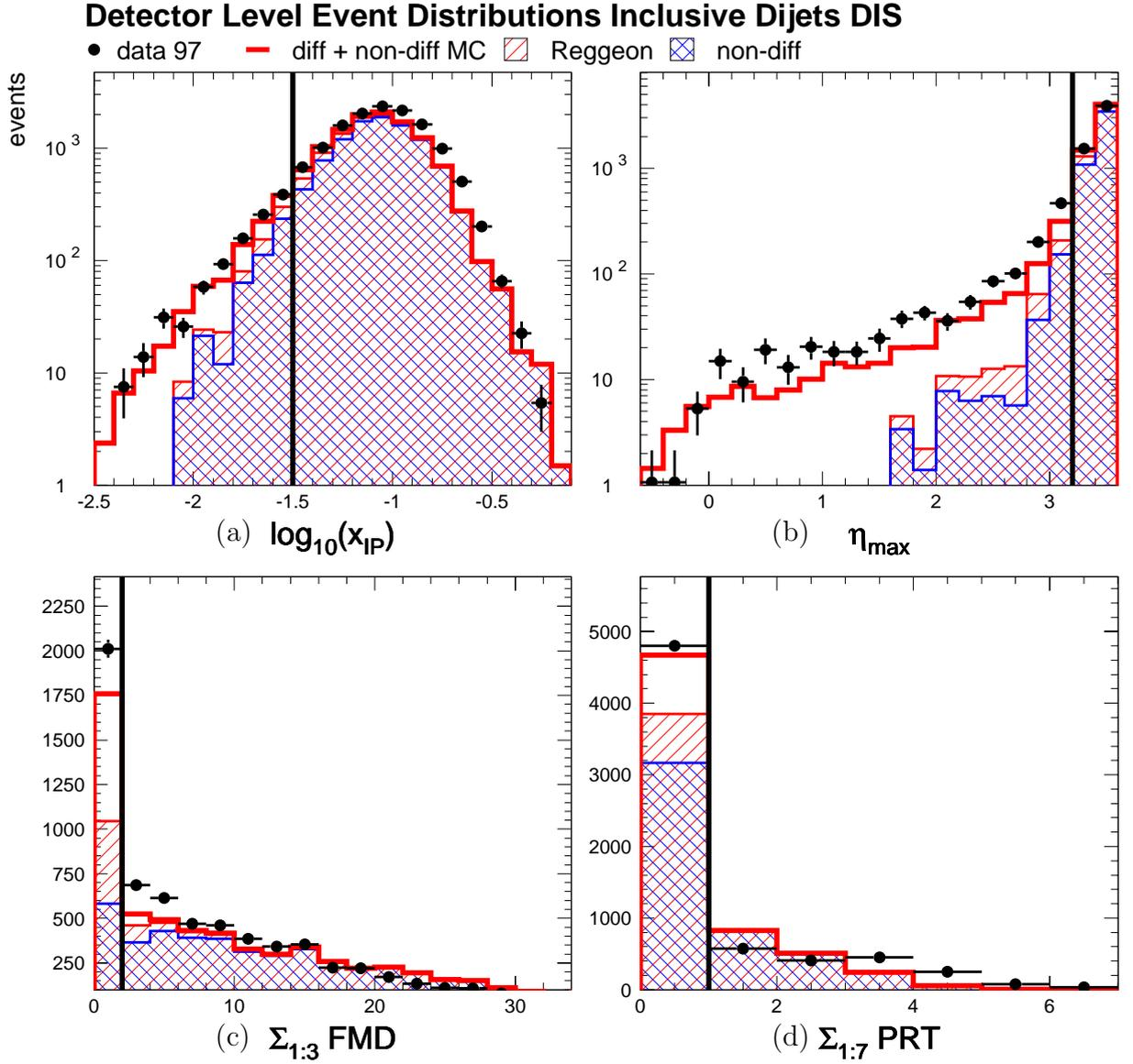
**Fig. 6.15.** Distributions of the diffractive cut variables for the events of the inclusive DIS dijet sample of 97. (a)  $x_P$ , (b)  $\eta_{\max}$ , (c) FMD and (d) PRT. For (c), FMD noise has been added in the MC.
