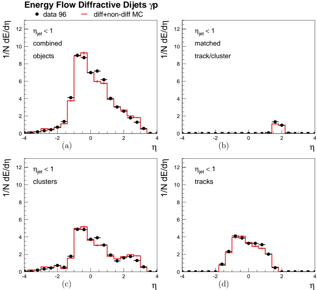
**Fig. 5.16.** Energy flow for the diffractive  $\gamma p$  dijet sample in 96. Shown is the mean energy as a function of the pseudorapidity  $\eta$  in the laboratory frame. The energy is reconstructed from (a) combined track and calorimeter cluster information, (b) only matched tracks and clusters, (c) clusters, and (d) tracks. The jets are required to satisfy  $\eta_{\text{jets}} < 1$ .
