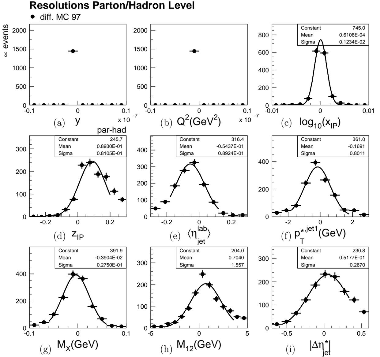
**Fig. 6.4.** Resolutions for reconstructing the parton level quantity at the hadron level. Shown is the difference between the variable as defined at the parton level and the variable reconstructed at the hadron level. The resolutions are evaluated with the diffractive MC for 97.
