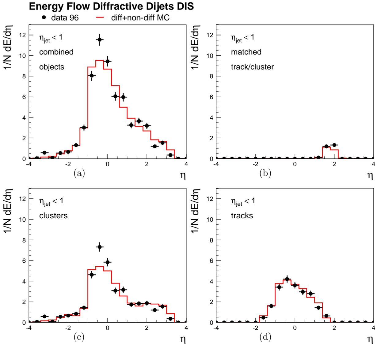
**Fig. 6.19.** Energy flow for the diffractive DIS dijet sample in 96. Shown is the mean energy as a function of the pseudorapidity  $\eta$  in the laboratory frame. The energy is reconstructed from (a) combined track and calorimeter cluster information, (b) only matched tracks and clusters, (c) clusters, and (d) tracks. The jets are required to satisfy  $\eta_{\text{jet}} < 1$ .
