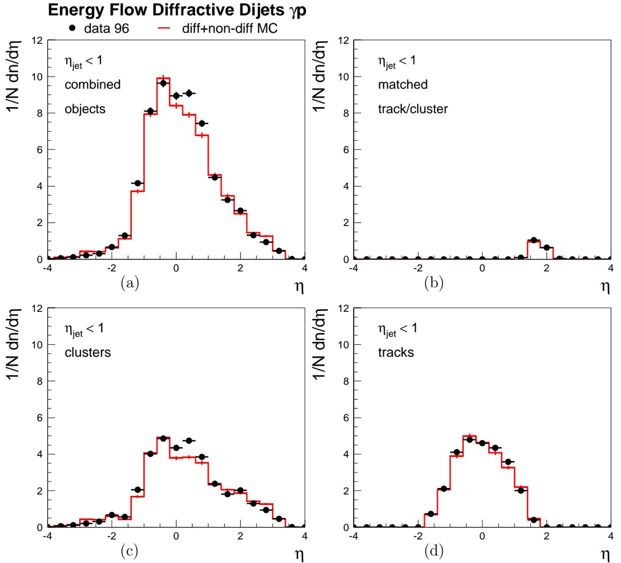
**Fig. 5.17.** Multiplicity for the diffractive  $\gamma p$  dijet sample in 96. Shown are as a function of the pseudorapidity  $\eta$  in the laboratory frame the average numbers of (a) combined objects from tracks and calorimeter clusters, (b) matched tracks and clusters, (c) clusters, and (d) tracks. The jets are required to satisfy  $\eta_{\text{jet}} < 1$ .
