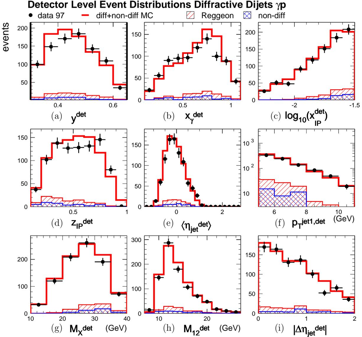
**Fig. 5.15.** Diffractive dijet photoproduction distributions for 97. The diffractive model is only reweighted in  $z_{\text{vtx}}$ . The number of MC events is normalised to the number of data events.
