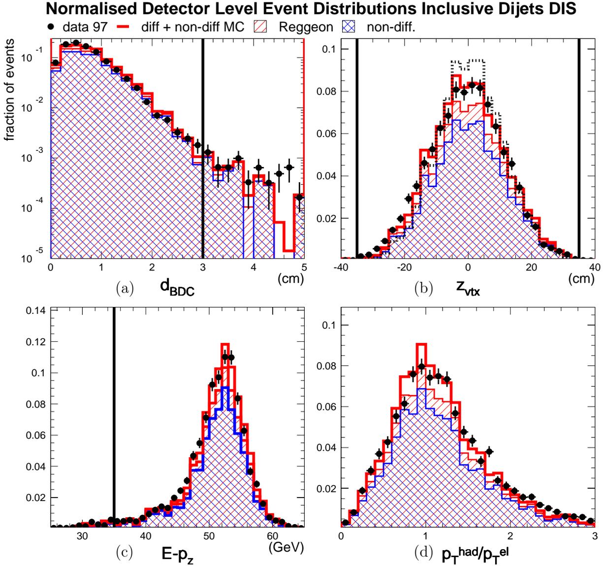
**Fig. 6.12.** Normalised distributions for the inclusive DIS dijet sample. (a) Distance between the electron cluster and the nearest track in the BCD. (b) The  $z_{\text{vtx}}$  distribution of the Monte Carlo has been reweighted. The original prediction is shown as the dotted histogram. (c) The quantity  $E - p_z$ . (d) The ratio of the transverse momenta of the electron and the hadronic system.
