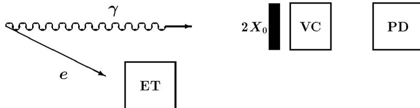
**Fig. 3.7.** Bethe Heitler Bremsstrahlung process as seen by the H1 luminosity system. The electron and photon are detected in the small angle electron detector ET and the photon detector PD, respectively. The PD is shielded from synchrotron radiation by a lead filter of two radiation lengths and a water Čerenkov counter.
