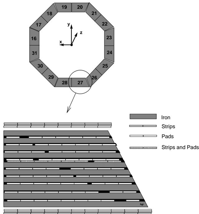
Figure 2.9: The structure of an Instrumented Iron module.
