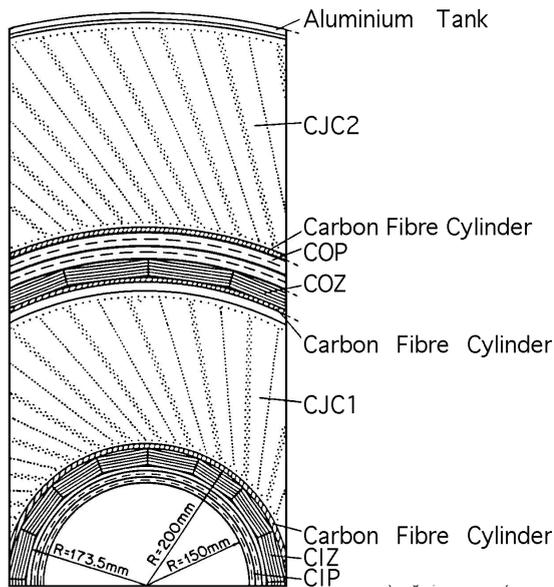
Figure 2.4: A cross sectional view of the Central Track Detector.
