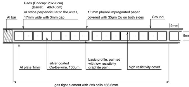
Figure 2.8: Cross-sectional structure of a layer of LST's.
