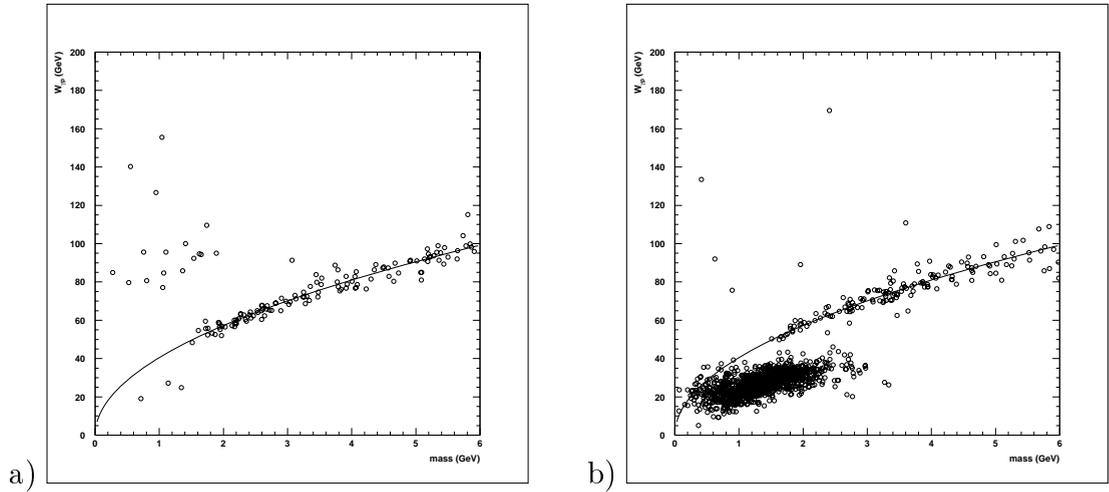
Figure 7.14:  $W_{\gamma p}$  vs. mass for a) electron beam on gas, and b) proton beam on gas, before analysis cuts. The curve is the expected relation for cosmic rays.
