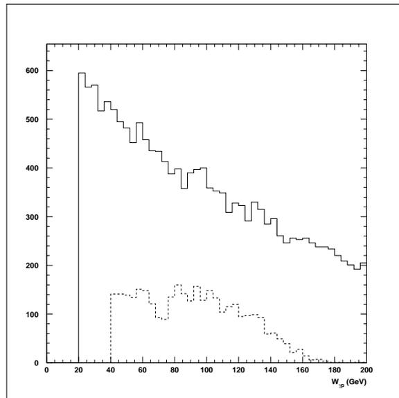
Figure 7.18:  $W_{\gamma p}$  distributions from DIFFVM Monte Carlo. The solid line is the generated distribution. The dashed line represents the effects of acceptance and selection efficiency.
