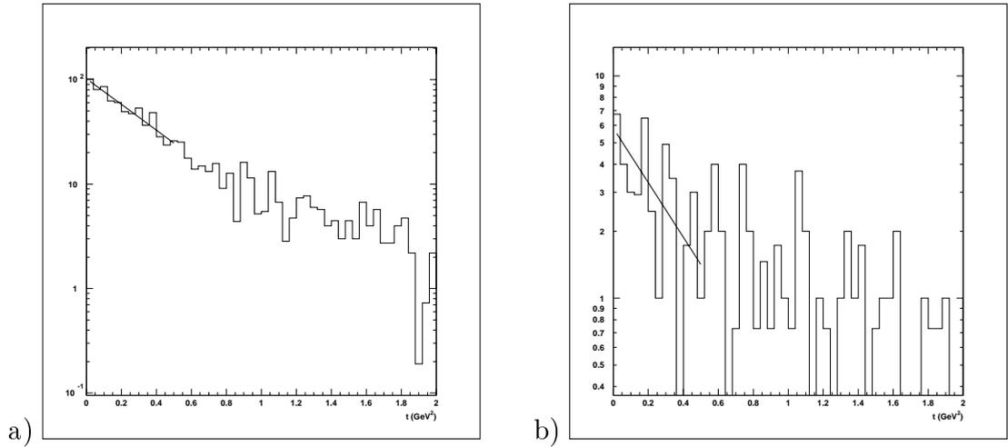
Figure 7.26: Dilepton  $t$  distribution for 1994 data, after analysis cuts and background subtraction, for a) standard event selection and b) dissociative event selection. The solid lines are exponential fits.
