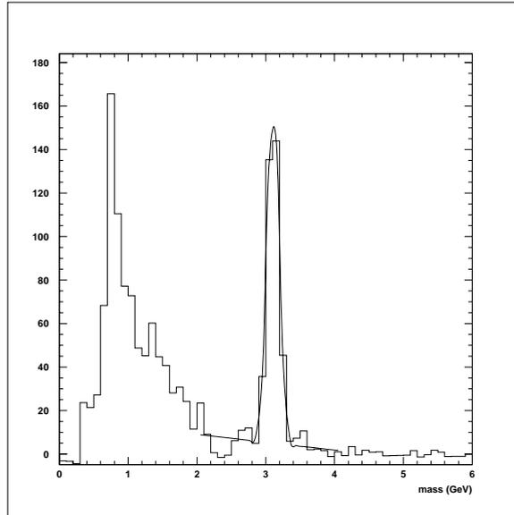
Figure 7.22: Mass of dimuon events triggered by the iron endcap subtrigger.
