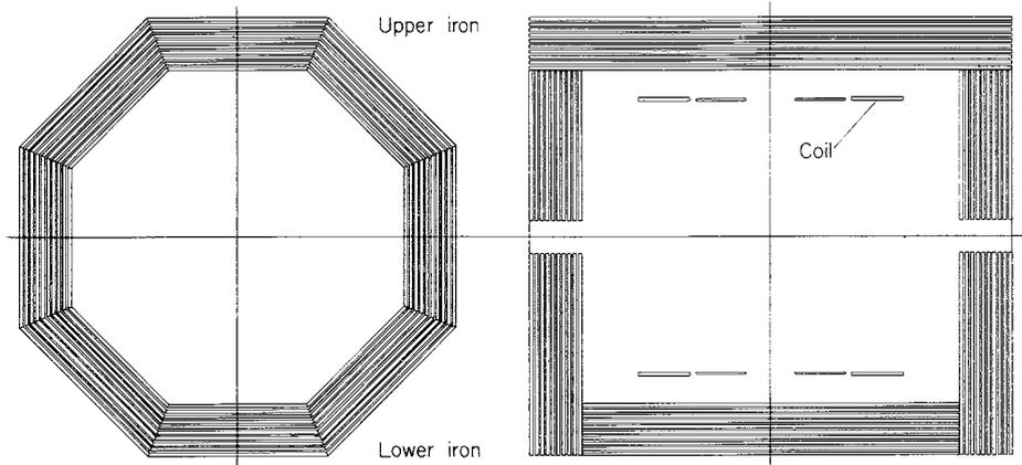
Figure 4.15: Radial (left) and side (right) views of the iron yoke.
