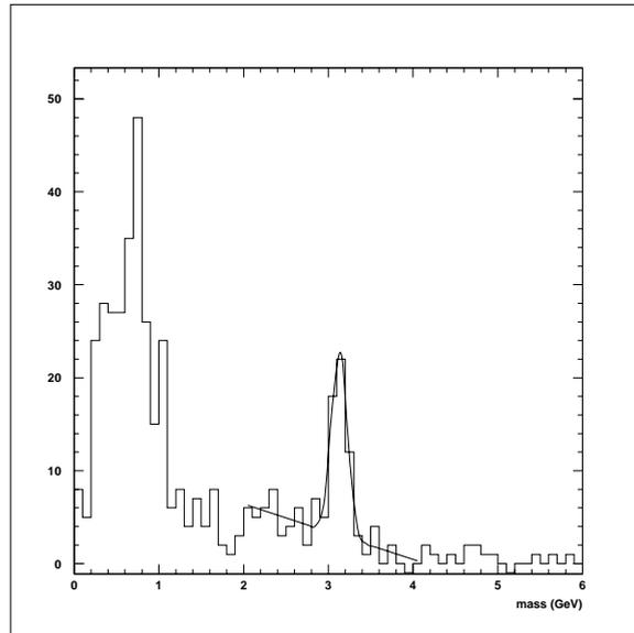
Figure 7.31: Dilepton mass distribution for the high- $Q^2$  event sample, after analysis cuts. The solid line is a fit of a gaussian plus a linear background.
