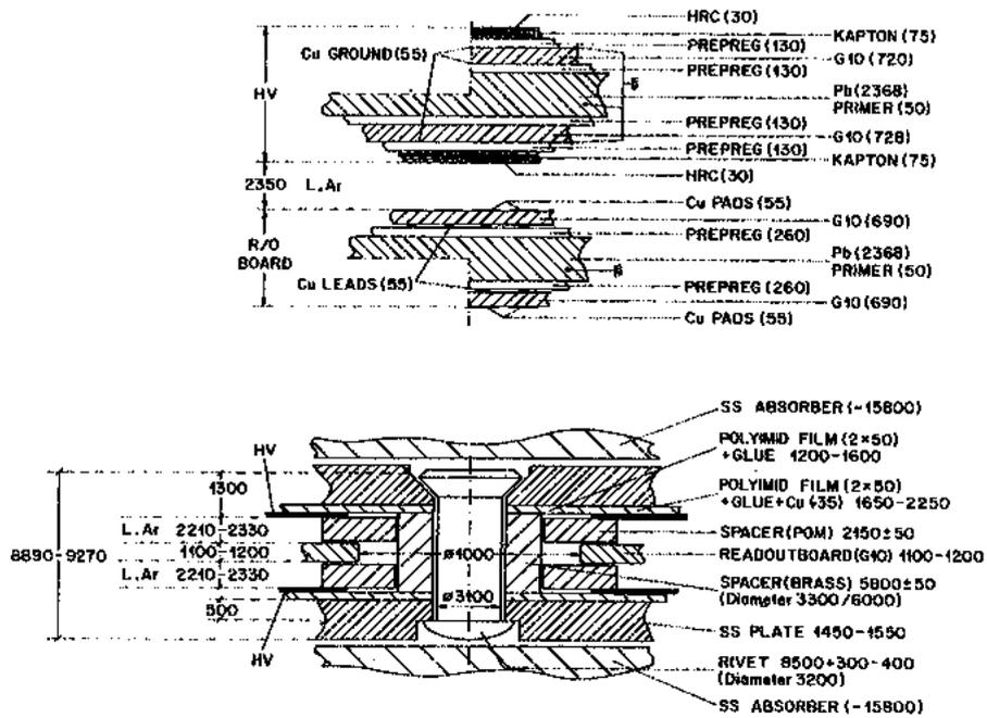
Figure 4.12: Schematic view of readout cell for electromagnetic (above) hadronic (below) sections of the LAr. All dimensions are in  $\mu\text{m}$ .
