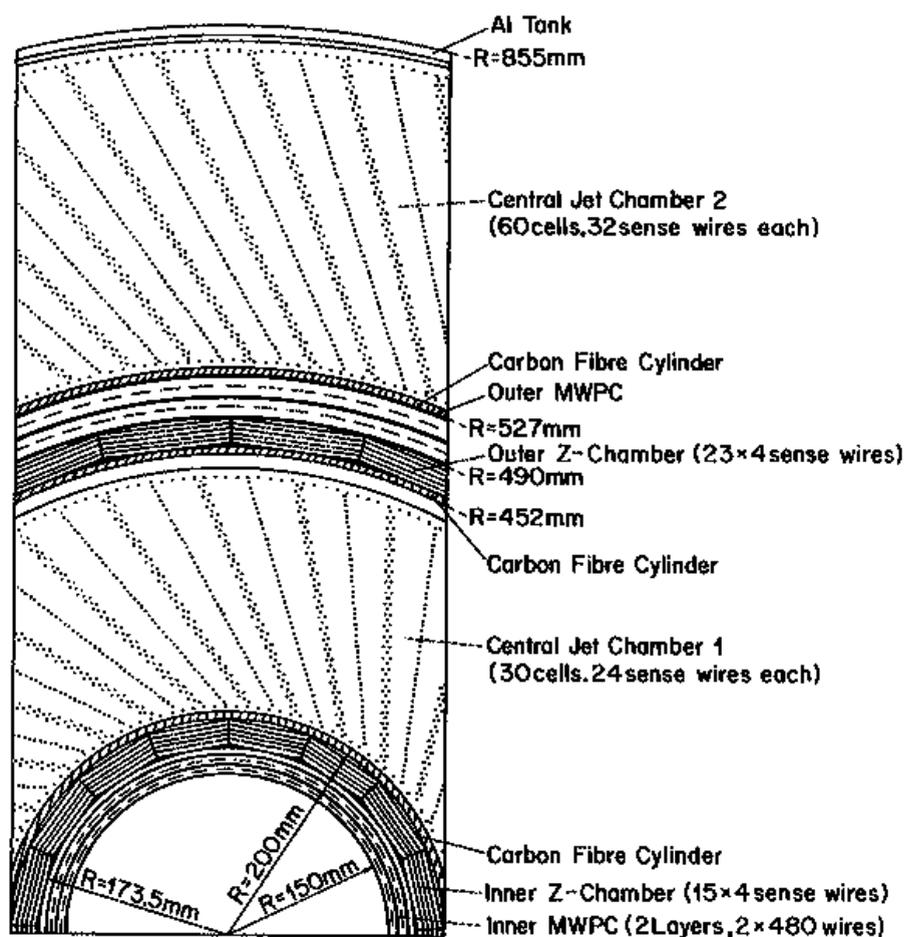
Figure 4.5: The central tracking system - radial view.
