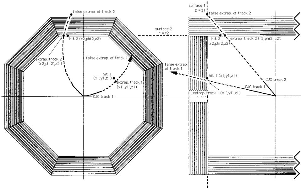
Figure 5.2: A demonstration of how tracks are extrapolated to the target surface of candidates. Note how the wrong combinations of track and candidate typically give very bad matches.
