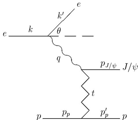
Figure 2.1: Feynman diagram for  $J/\psi$  production showing four-momenta.
