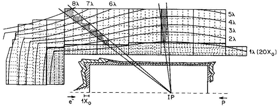
Figure 4.11: Iso- $X_0$  and iso- $\lambda$  lines for the LAr calorimeter, including the material of the trackers and the cryostat wall (hashed areas). The dashed lines indicate the segmentation of the calorimeter.
