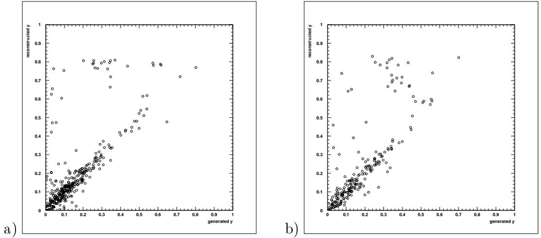
Figure 6.7: Reconstructed vs. generated  $y$  for high- $Q^2$  a) elastic events, and b) proton dissociative events from the DIFFVM Monte Carlo.
