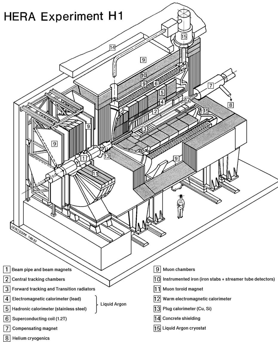
Figure 4.1: The H1 Detector at HERA - cutaway view.
