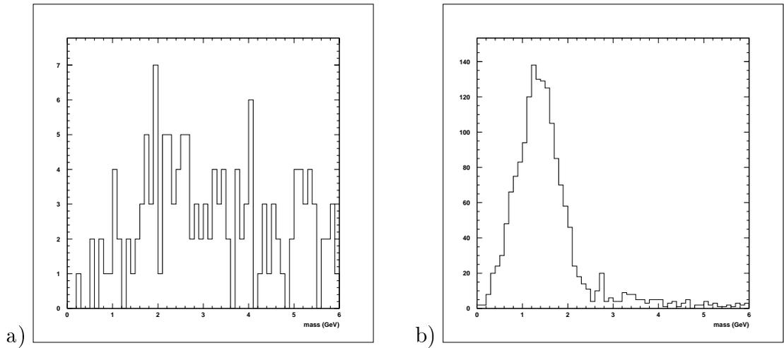
Figure 7.12: Mass distributions for a) electron beam on gas, and b) proton beam on gas, before analysis cuts.
