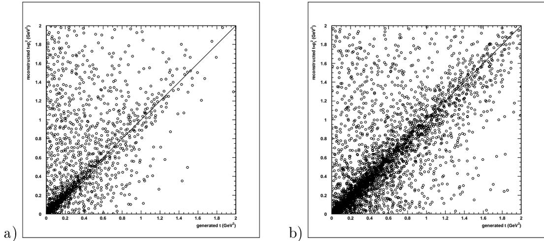
Figure 6.5: Reconstructed vs. generated  $t$  for a) elastic events, and b) proton dissociative events from the DIFVIM Monte Carlo.
