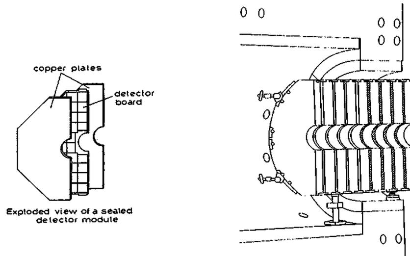
Figure 4.14: View of the plug calorimeter, showing exploded view of single module (left), and entire subdetector (right).
