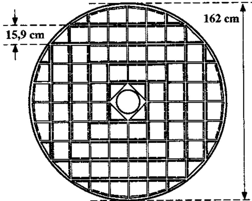
Figure 4.13: Radial view of the BEMC.
