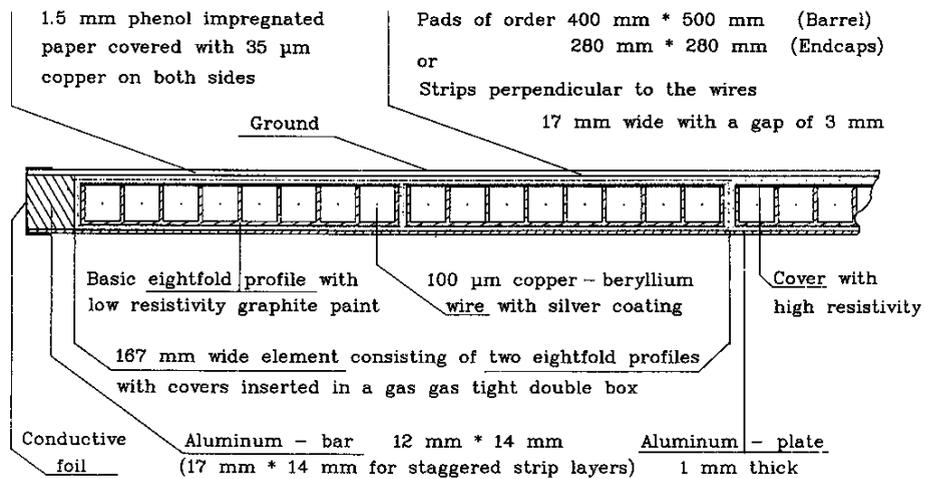
Figure 4.16: Construction of a limited streamer tube module.
