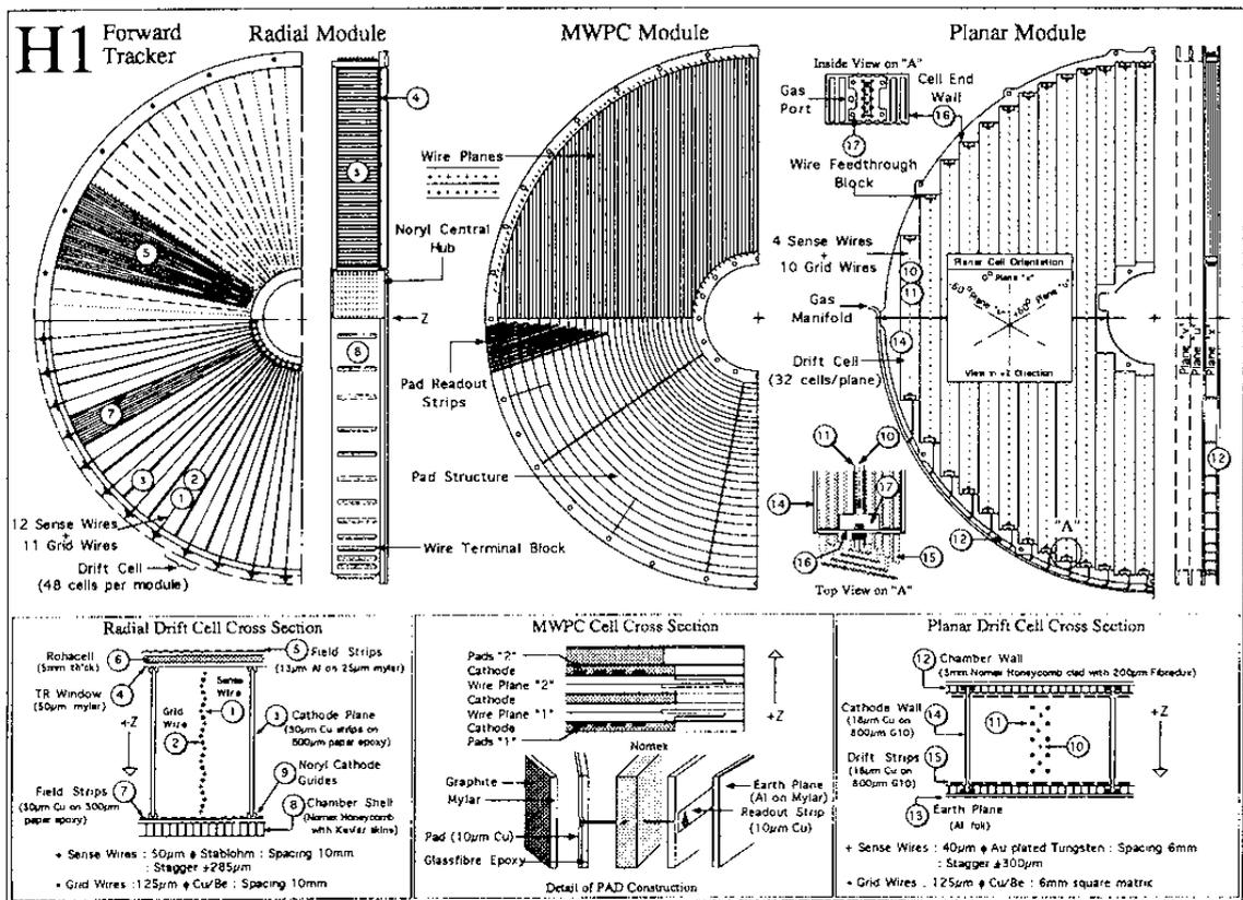
Figure 4.8: Detailed view of the construction of the supermodule components. Above are the radial and side views, and below are cell cross sections.
