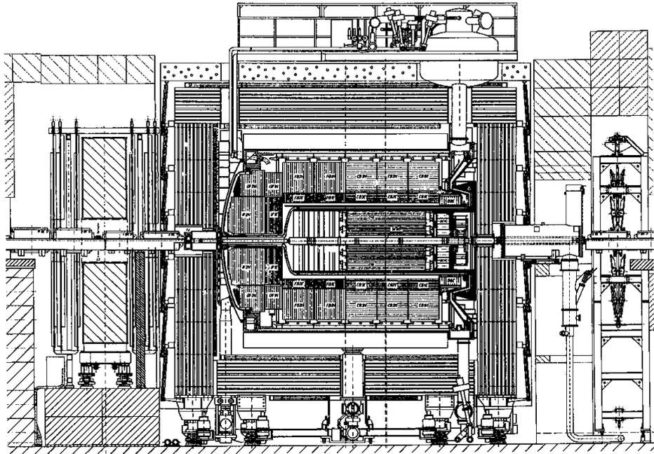
Figure 4.2: The H1 Detector at HERA - side view.
