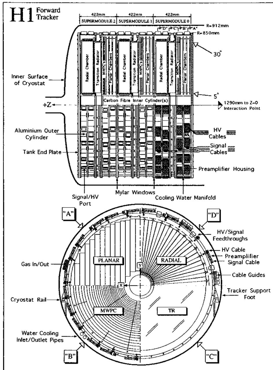
Figure 4.7: Layout of the forward tracker. Above is a side view of the supermodules, and below is a radial view showing the cell structure of the supermodule components, one per quadrant.
