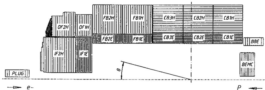
Figure 4.9: Side view of the liquid argon calorimeter showing LAr wheels, as well as plug and BEMC.
