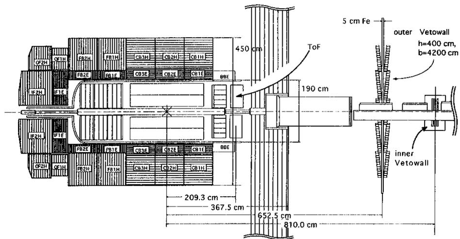
Figure 4.17: Side view showing the location of the TOF and veto walls with respect to the main detector.
