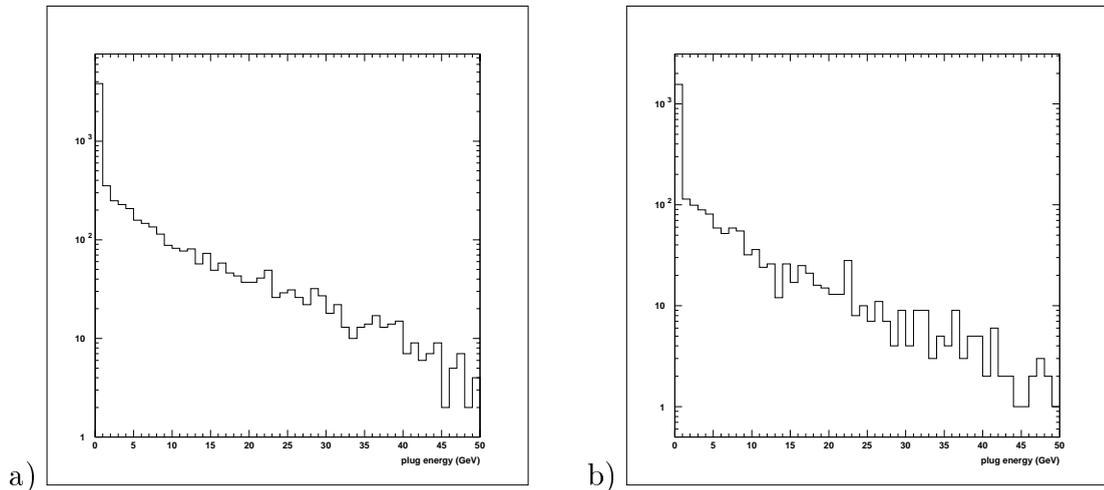
Figure 7.19: Plug energy for proton dissociative events from the DIFFVM Monte Carlo a) before analysis cuts and b) after analysis cuts.
