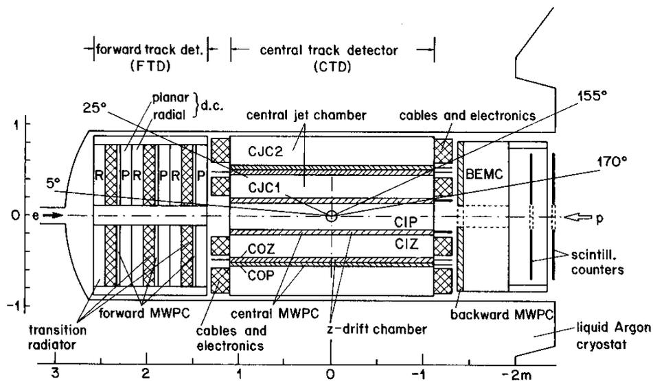
Figure 4.4: The H1 tracking system - side view.
