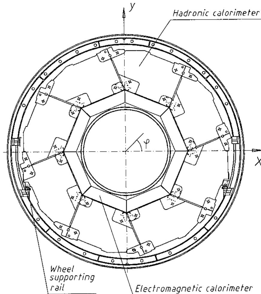
Figure 4.10: Radial view of the liquid argon calorimeter.
