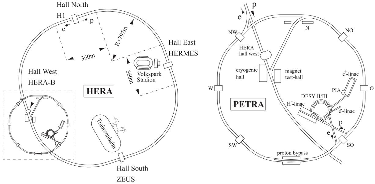
Figure 1.1: Layout of HERA and its pre-accelerators.
