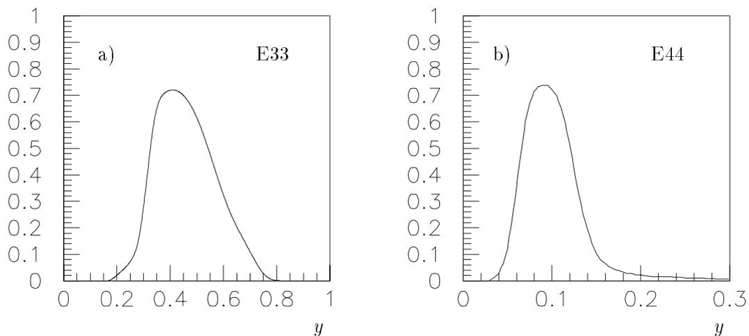
**Figure 4.11:** Acceptance function of the electron taggers during one run range. a) E33, b) E44.
