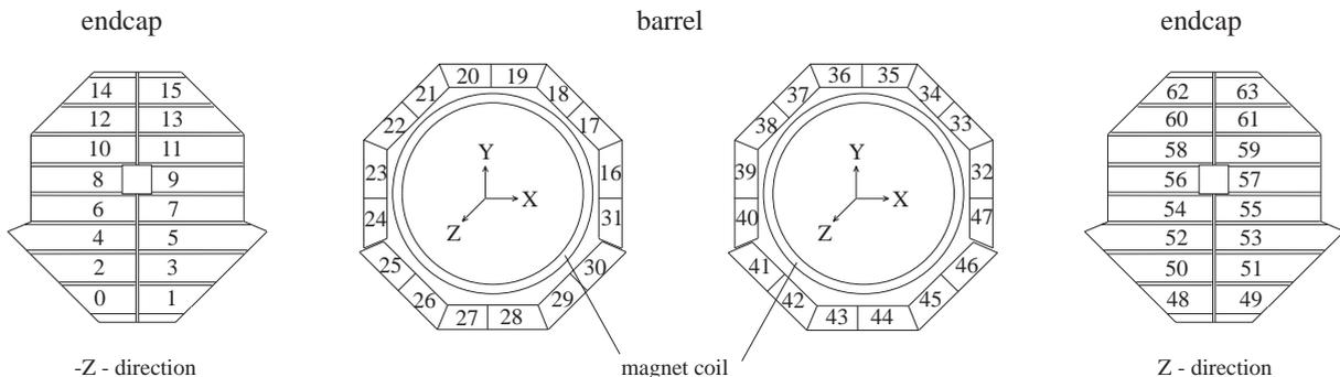
**Figure 1.4:** The 64 modules of the instrumented iron. The instrumented iron detects muons and is used as a return yoke for the magnetic field from the superconducting coil. Modules 6...11 (54...59) belong to the inner backward (forward) endcap.
