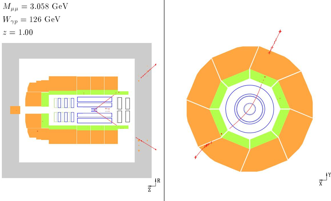
**Figure 4.2:** Schematic display of a candidate event for elastic  $J/\psi$  meson production. A side view of the H1 detector is shown at the left and a radial view of the central drift chambers and the LAr calorimeter at the right. Both muons were identified in the instrumented iron and no other particles were registered.
