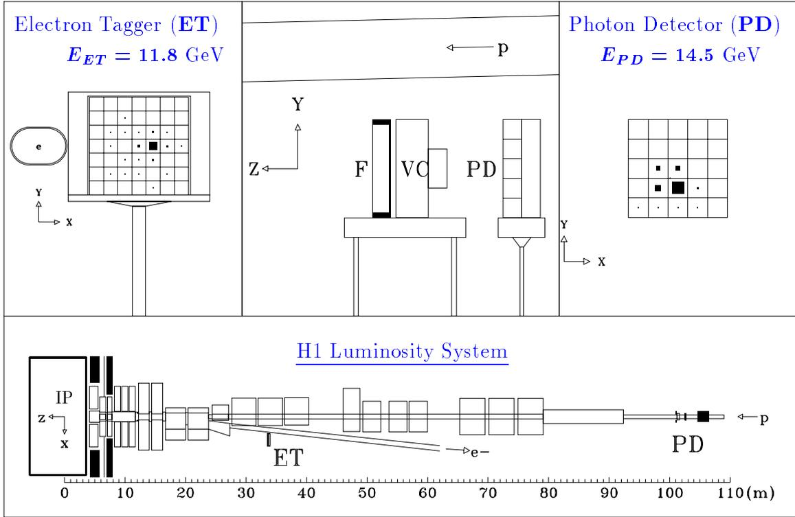
**Figure 1.5:** A Bethe-Heitler bremsstrahlung event measured with the luminosity system. The electron deposits  $E_e = 11.8$  GeV in the electron tagger E33 (upper left), while the photon energy  $E_\gamma = 14.5$  GeV is measured in the photon detector (PD, top right). The lower part shows a top view of the luminosity system. The middle part shows details of the photon detection system. F is a lead absorber and VC a water Cherenkov veto counter.
