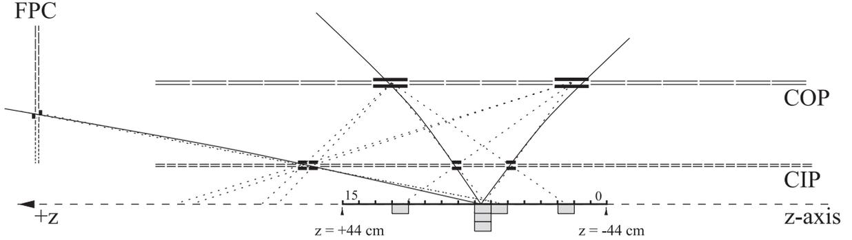
**Figure 1.6:** Principle of operation of the z-Vertex Trigger. The side view shows an event with three tracks originating from genuine particles (solid lines). The dotted lines represent all possible combinations of CIP, COP and FPC hits. The z-Vertex histogram shows a maximum at the  $z$  position of the primary event vertex.
