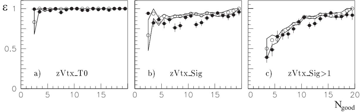
**Figure 4.10:** Efficiency of the  $z$  Vertex histogram trigger elements a)  $zVtx\_T0$  b)  $zVtx\_Sig$  and c)  $zVtx\_Sig>1$  as a function of the number of good tracks in data (full points) and Monte Carlo (open points) before correction. The statistical error of the Monte Carlo efficiency is shown as a band.
