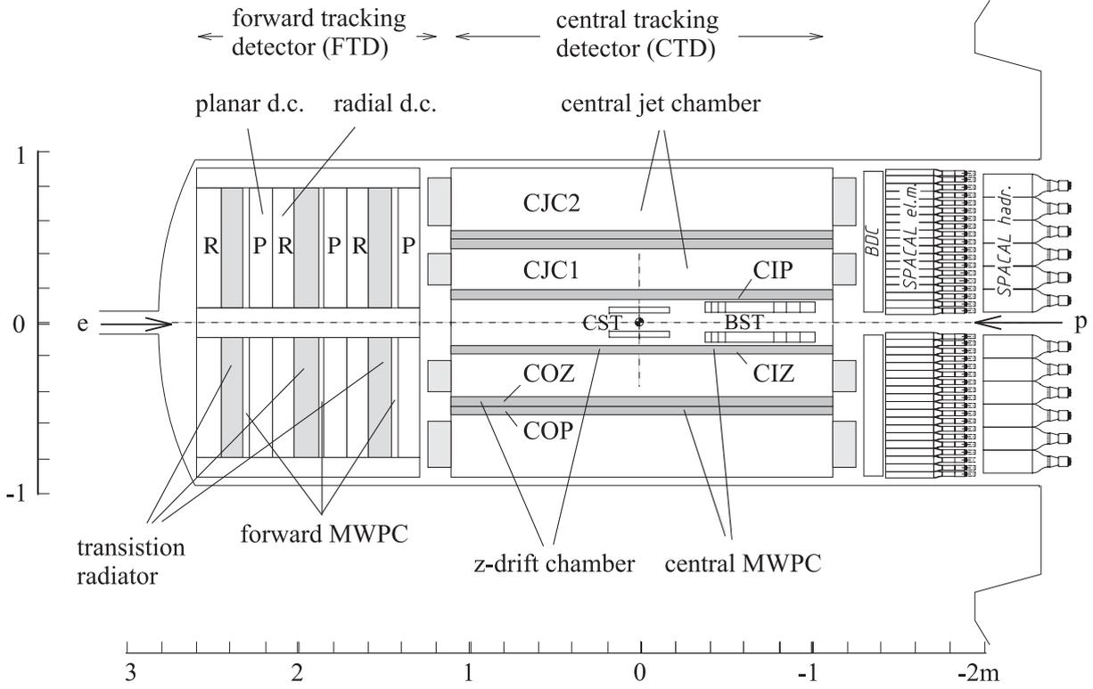
Figure 1.3: Side view of the tracking chambers.
