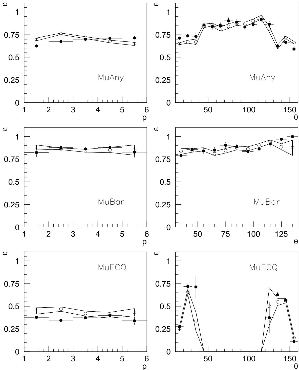
**Figure 4.9:** Efficiencies of the instrumented iron's trigger elements in data (full points) and Monte Carlo simulation (open points) as a function of the muon's momentum  $p$  and polar angle  $\theta$ . The statistical error of the Monte Carlo efficiency is shown as a band.
