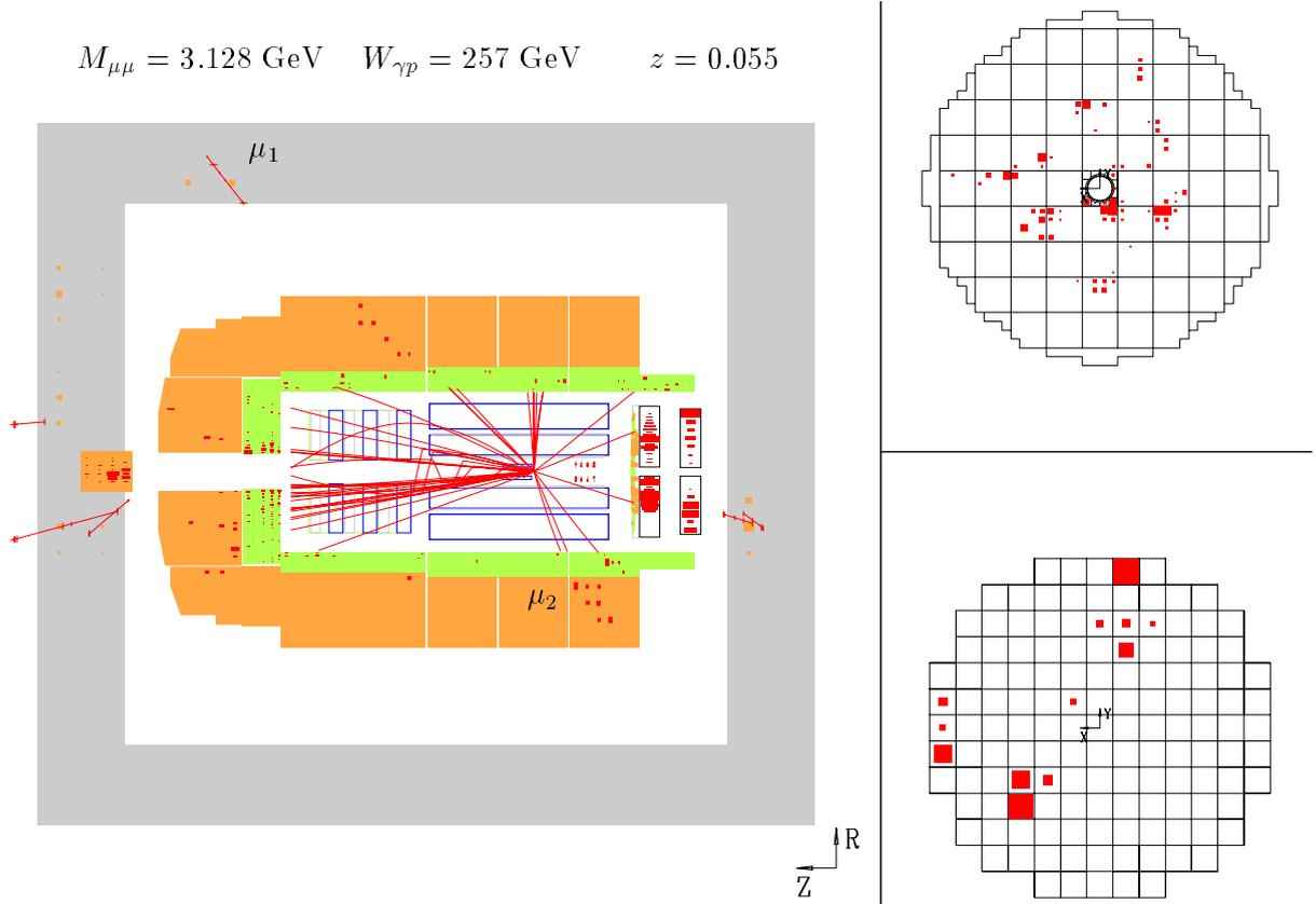
**Figure 4.1:** Schematic display of a candidate event for  $J/\psi$  meson production in a resolved photon process. A side view of the H1 detector is shown at the left and a radial view on the backward calorimeter at the right. One muon was identified in the instrumented iron, the other muon in the calorimeter. A wide spread energy deposition (most likely produced from the remnants of the photon) can be seen in the electromagnetic (top) and hadronic Spacal (bottom).
