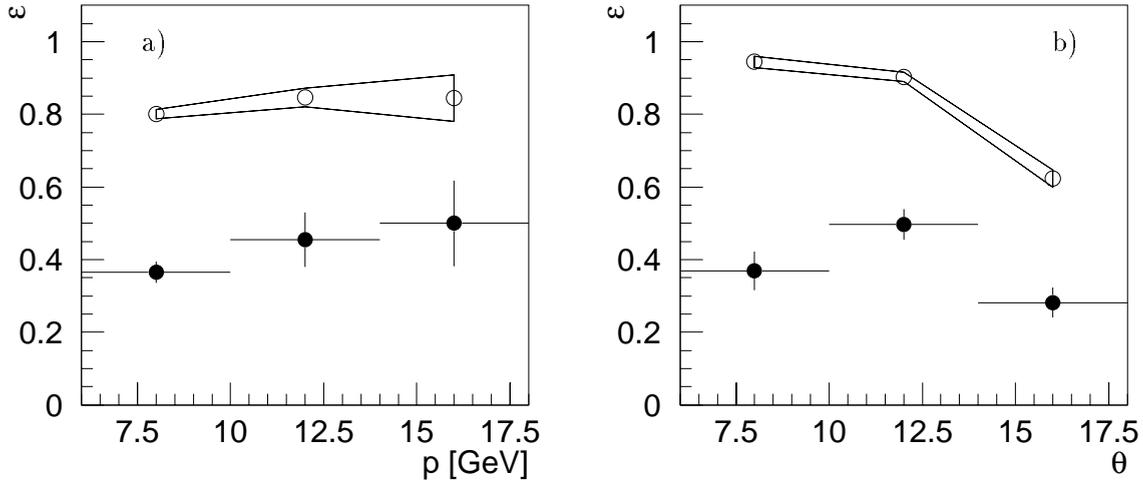
**Figure 3.7:** Reconstruction efficiency of the forward muon detector in data (full points) and Monte Carlo (open points) as a function of *a*) the muon's momentum  $p$  (integrated over  $6^\circ < \theta < 18^\circ$ ) and *b*) its polar angle  $\theta$  (for  $p > 6$  GeV). The statistical error of the Monte Carlo efficiency is shown as an error band.
