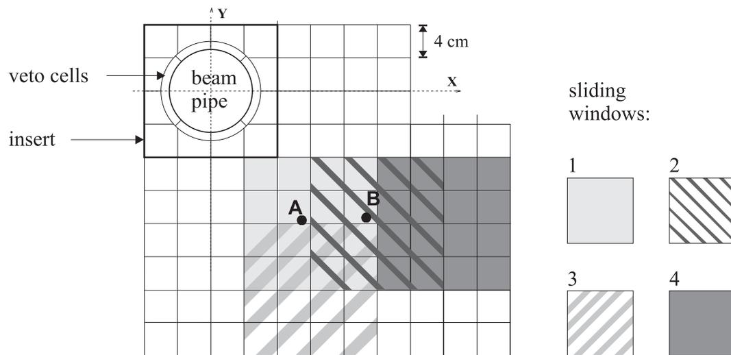
**Figure 1.7:** Principle of operation of the Spacal IET trigger. The total energy of a cluster around point A (B) will be collected in sliding window 1 (2). The trigger fires if at least one sliding window exceeds a predefined energy threshold.
