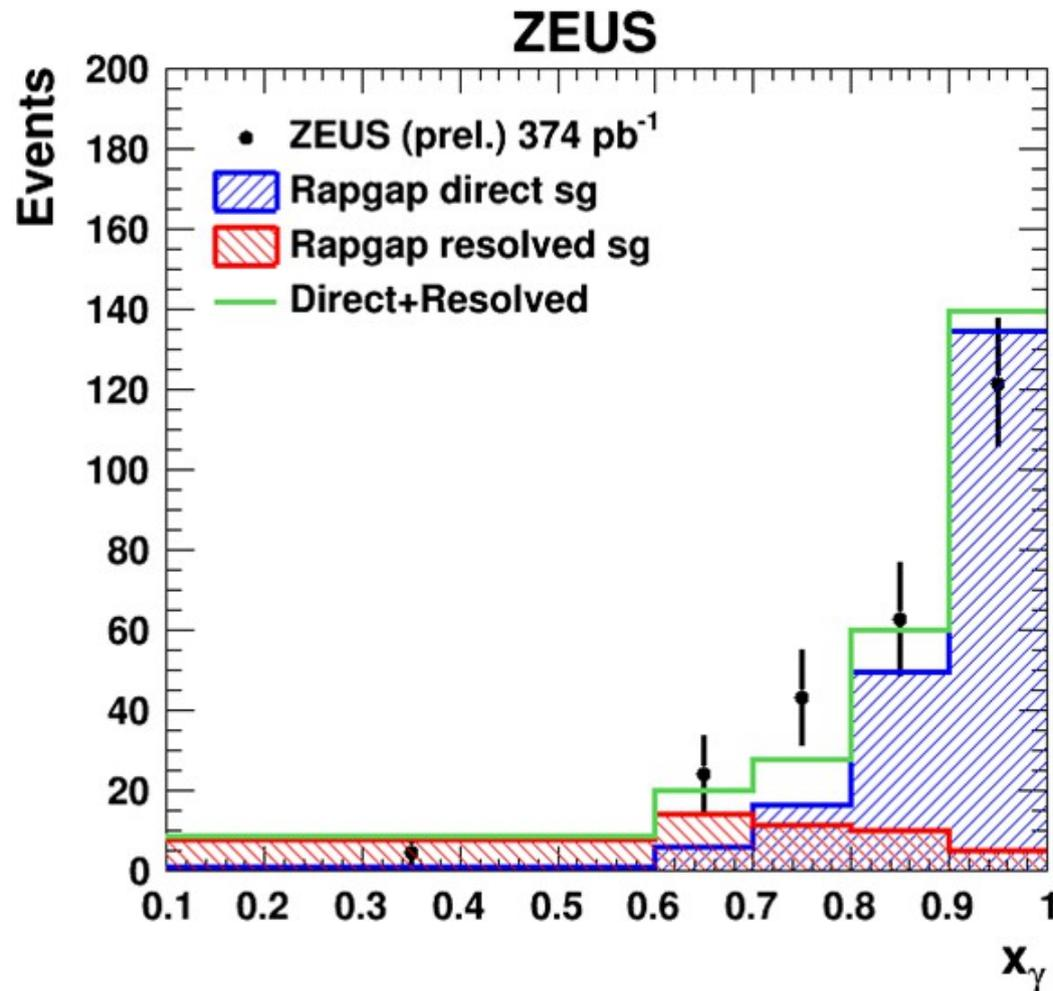
$$x_\gamma = \frac{\sum_{\gamma + \text{jet}} (E - p_z)}{\sum_{\text{all EFOs}} (E - p_z)}$$
