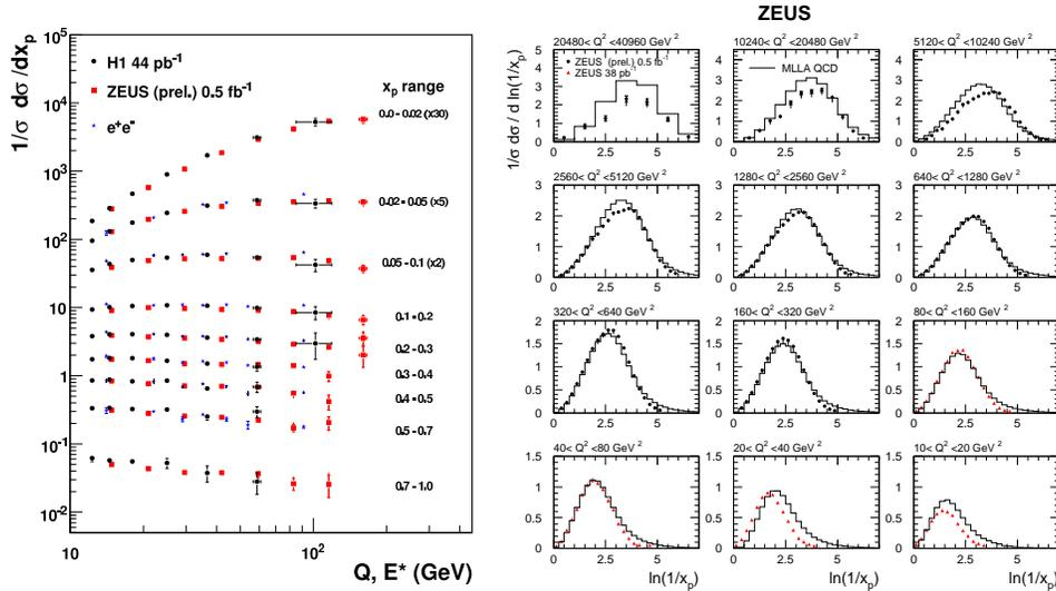
Figure 3: Left: the charged particle distribution shown as a function of  $Q^2$  in  $x_p$  bins; similar measurements from  $e^+e^-$  are overlaid. Right: the normalized  $\ln(1/x_p)$  distributions shown as the black dots for different  $Q^2$  intervals; the full line represents the MLLA+LPHD predictions.
