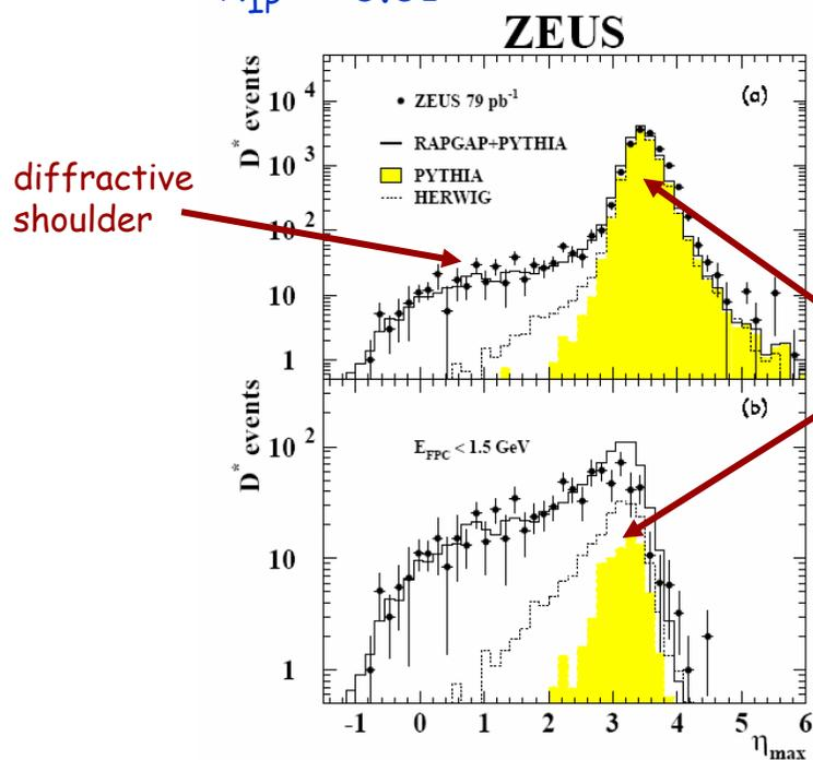
Strong reduction of non-diffractive background by cut on forward plug calorimeter (FPC).
