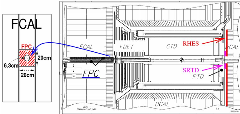
Forward Plug Calorimeter (FPC):
