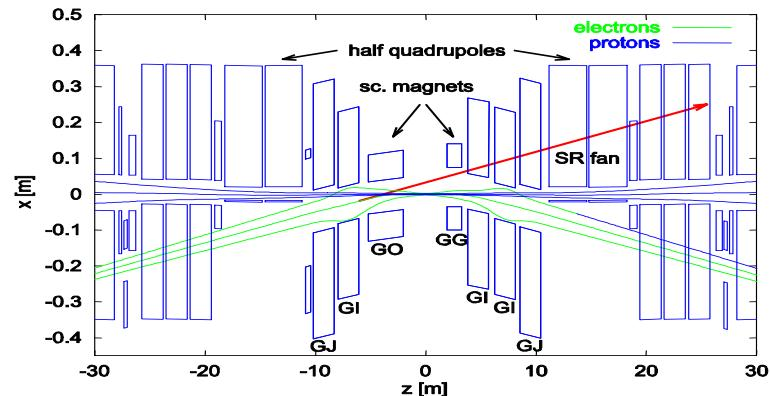
**“mini-beta” final focusing magnets closer to detector**
