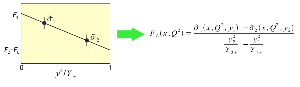
larger y difference more points (beam energies)  $\Rightarrow$  higher accuracy of  $F_{L}$  measurement
