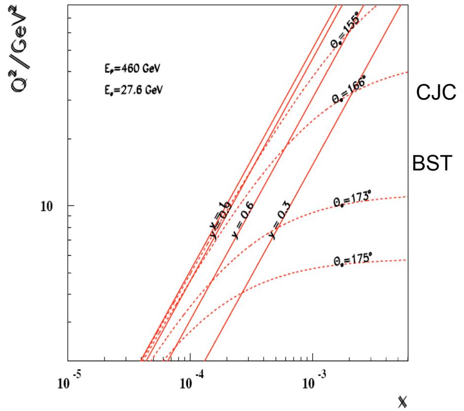
The low  $Q^2$  acceptance limit is given by the high  $E_p$ , **large theta cut - inner radius of SPACAL,  $\sim 173^\circ$** .
