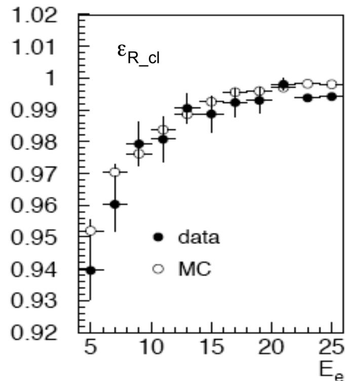
Drop of cut efficiency for  $R_{cluster} < 4\text{cm}$  as measured with tagged ISR events,  $\Sigma E > 22\text{ GeV}$ , due to shower broadening and overlap of electron with soft FSR photon --> shower library to improve simulation.
