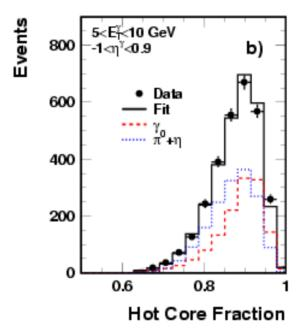
Likelihood discriminator used in  $(E_T, \eta)$  bins to allow for energy dependence and varying calorimeter granularity.
