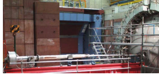
Figure 3. The 3.20 m long GO magnet attached to the beam pipe before insertion into the LAr cryostat of the H1 detector.
