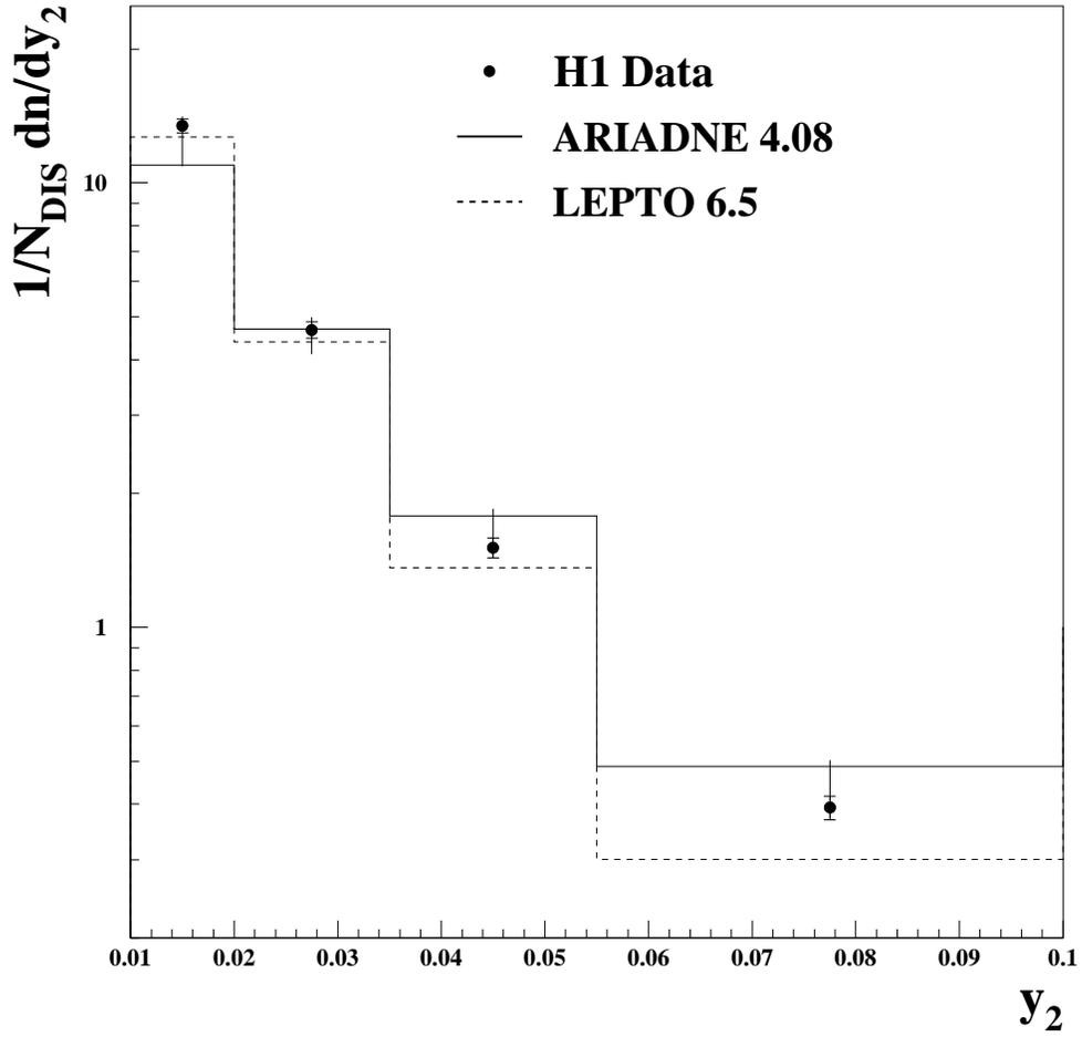
Figure 2: Distribution of the observable  $y_2$  corrected for detector effects compared with the prediction of the models ARIADNE 4.08 and LEPTO 6.5. As in Figure 1, the cut  $10^\circ < \theta_{jet} < 145^\circ$  is applied. The error bars correspond to the statistical and systematic errors added in quadrature. The inner error bars give the statistical error only.
