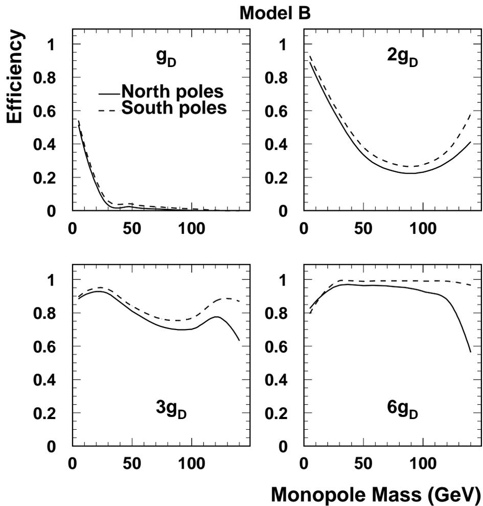
Figure 9: The efficiency for stopping monopoles of strength  $g_D$ ,  $2g_D$ ,  $3g_D$  and  $6g_D$  or more computed according to the monopole pair production model B.
