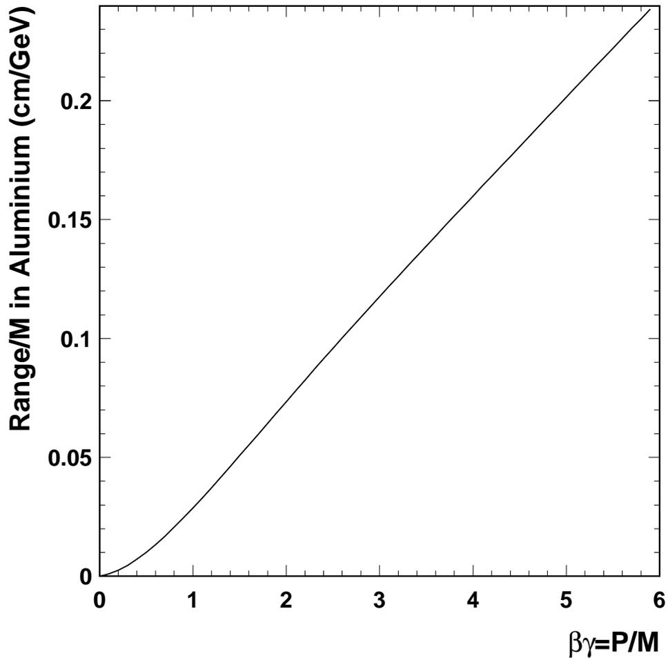
Figure 7: The ratio of the range to mass of a monopole of charge  $g_D$  in aluminium versus  $\beta\gamma$ . The range was calculated from the stopping power,  $dE/dx$ , in Fig. 1 of [28], adjusted to the electron density in aluminium.
