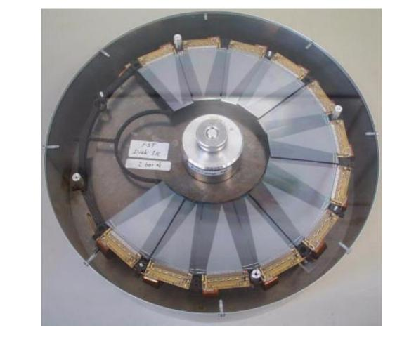
The new Forward Silicon Tracker (FST) consists of 12 single-sided silicon planes measuring tracks in 3 projections in the range from 7° to 17°. A radial plane shown here has 640 strips between 6 and 12 cm radius. The elliptical and excentric beam pipe accommodates only 12 of 16 azimuthal sectors.
