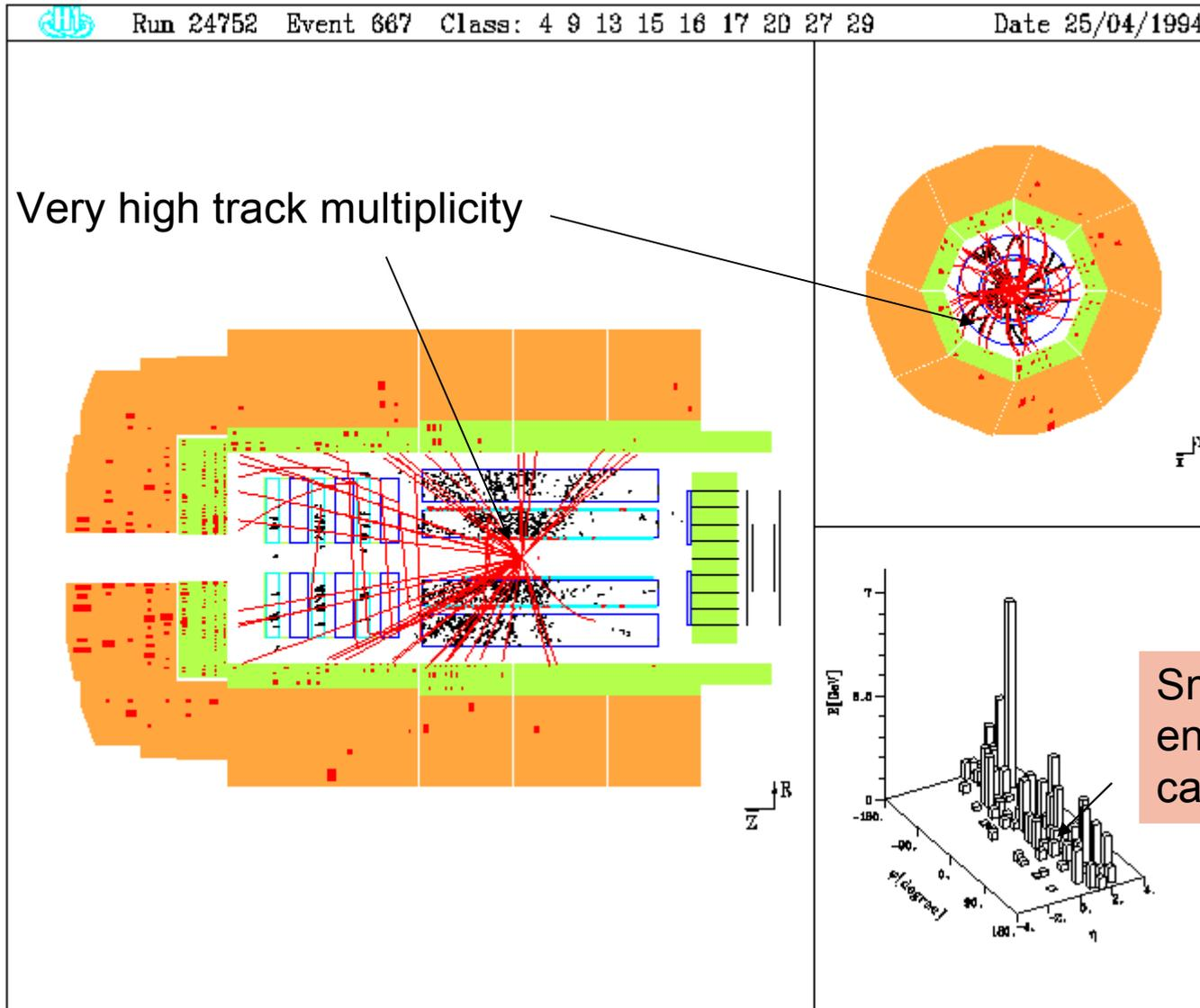
The Central Silicon Detector (CST) measures hits very precisely (10 micrometer).
