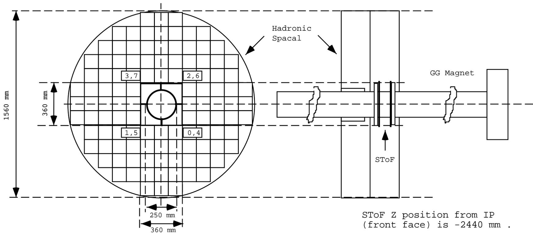
SToF consists of 2 layer plastic scintillating counters, installed around beam pipe inside of Hadronic Spacal. Each layer has 4 separated equal size counters, covered from one side with 1 mm Lead (black line on figure shows Lead covered side). Numbering of counters is also shown, where first and second layer corresponding numbers are divided by comma. The distance between layers is 110 mm. The thickness of plastic scintillator is 10 mm.
