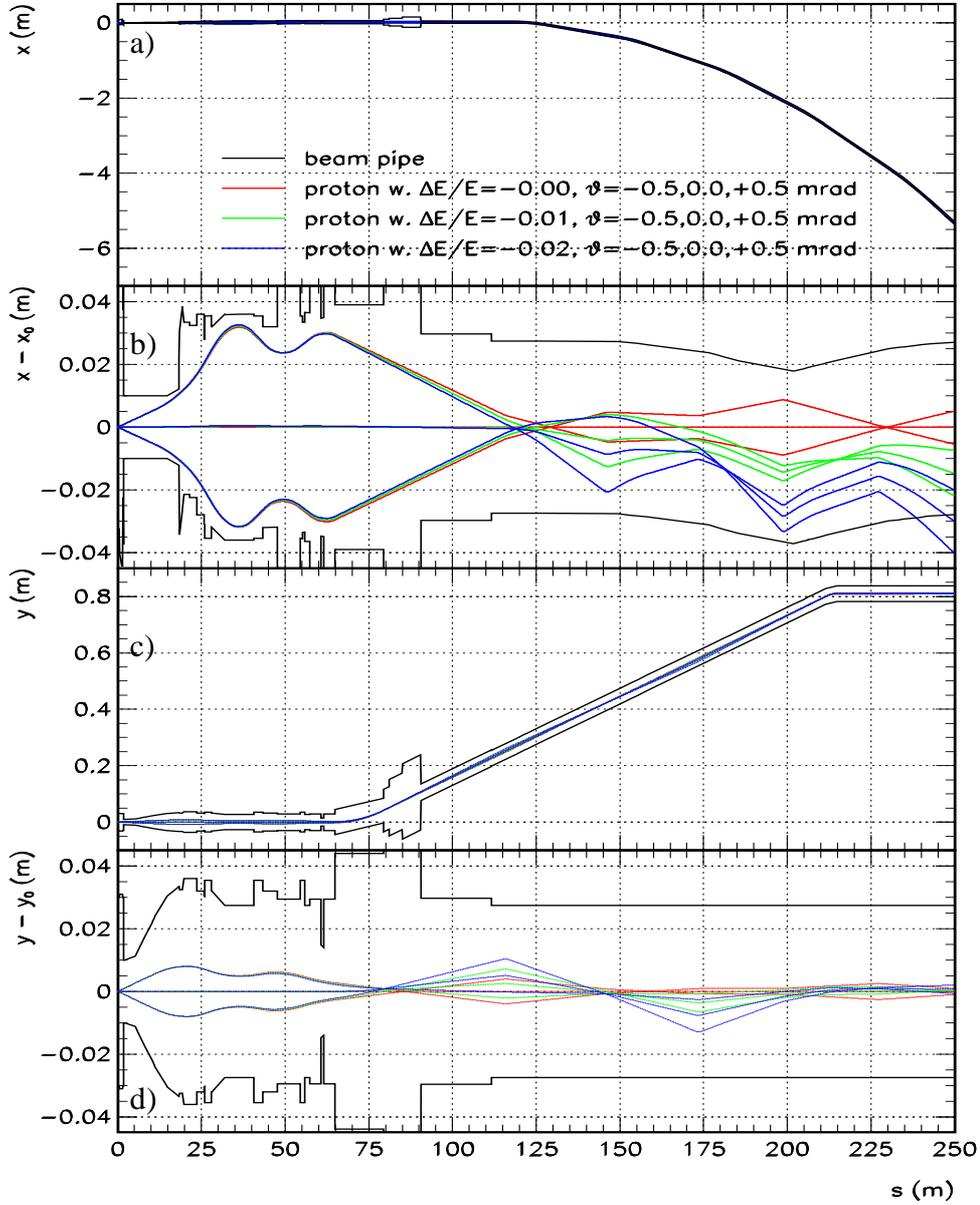
Figure 1: Horizontal and vertical projection of the beam pipe: a)  $x$ -projection of the proton beam pipe with respect to the absolute H1 coordinate system; b)  $x$ -projection of the beam pipe relative to the nominal beam position; c)  $y$ -projection of the proton beam pipe with respect to the absolute H1 coordinate system and d)  $y$ -projection of the beam pipe relative to the nominal beam position. Coloured lines show proton trajectories for given proton energy losses and emission angles.
