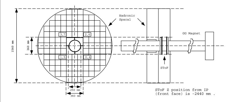
SToF consists of 2 layer plastic scintillating counters, installed around beam pipe inside of Hadronic Spacal. Each layer has 4 separeted equal size counters, covered from one side with 1 mm Lead (black line on figure shows Lead covered side). Numbering of counters is also shown, where first and second layer corresponding numbers are divided by comma. The distance between layers is 110 mm. The thickness of plastic scintillator is 10 mm.
