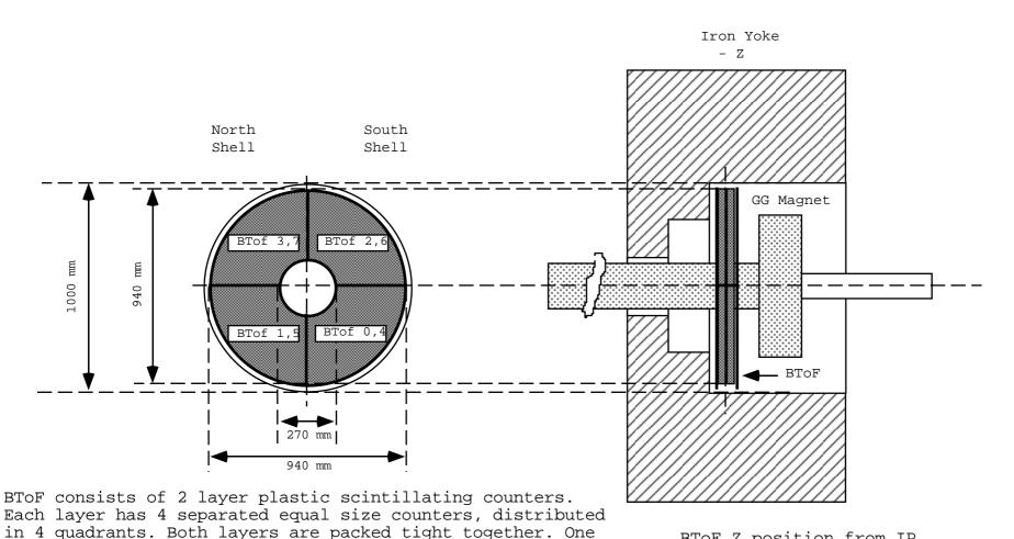
half of BTof is installed on South and second half on North
